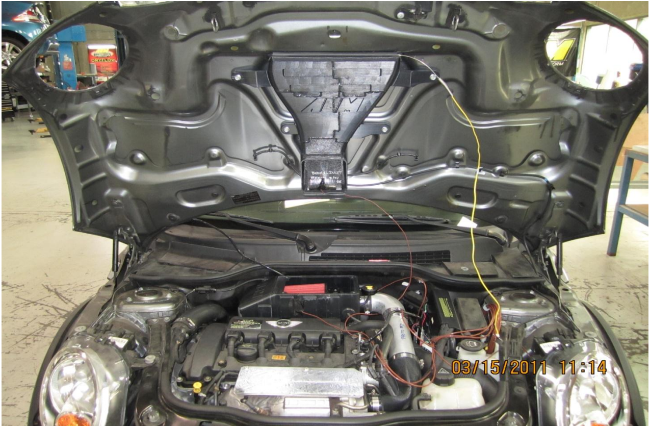
Figure1: Rapid Prototype AEM Intake with Cold-Air Hood Scoop instrumented with thermocouples for temperature testing:
