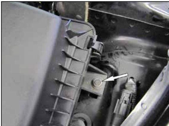
3. Remove the bolt that secures the air filter housing assembly to the inner fender and then remove the air filter housing from the vehicle.
