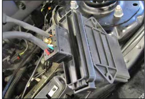
9. Route the K&N® wiring harness towards the driver's side inner fender and connect it to the boost module.
