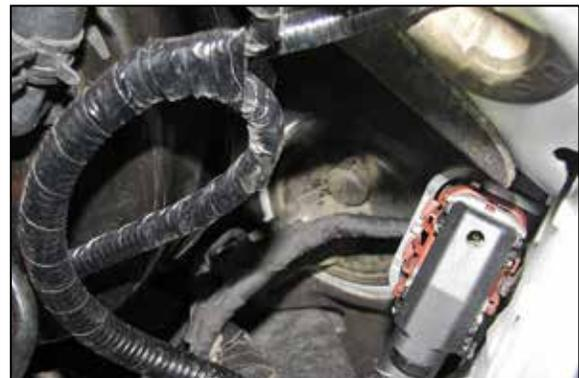
6. Create a small hole in the fire wall grommet and route the pedal harness through the hole into the engine compartment.
