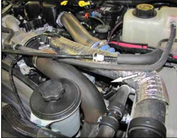
2. Locate the Fuel rail pressure sensor under the intercooler tube on the driver's side of the engine. Release the red locking tab and disconnect the factory wiring harness from the sensor.
