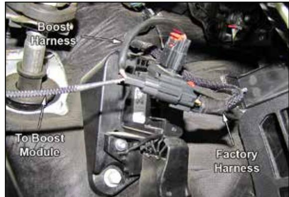
5. Connect the provided pedal harness into the factory harness and to the pedal assembly.
