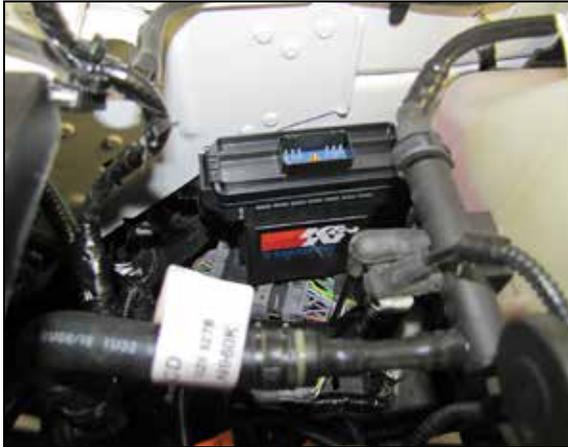
7. Secure the Boost module to the inner fender using the provided tie wraps.
