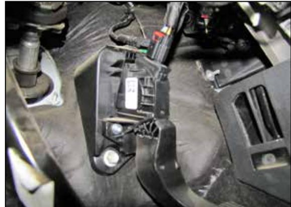
4. Locate the throttle pedal connector under the instrument panel. Release the red locking tab and disconnect the connector from the pedal assembly.
