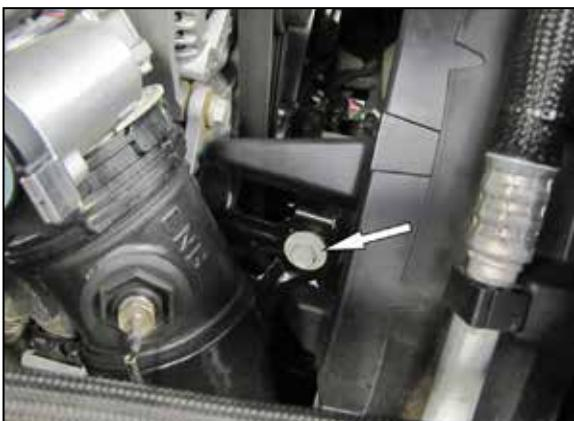
4. Remove the intake charge pipe mounting bracket bolt.
