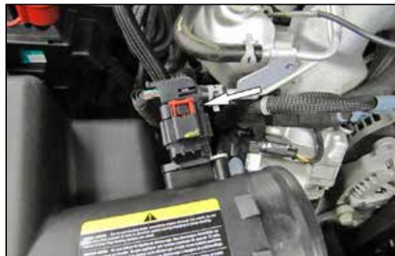
11. Reinstall the air filter housing so that the mounting studs insert into the mounting grommets. Reconnect the mass air sensor electrical connection.
