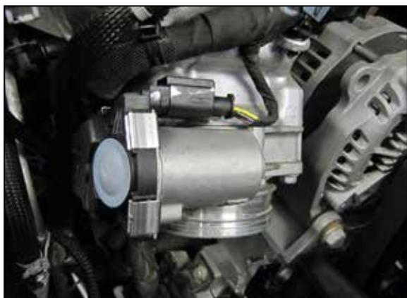
6. Disconnect the throttle body electrical connection and then remove the four bolts that secure the throttle body to the charge manifold. Remove the throttle body and gasket from the engine.
