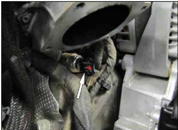
7. Locate the Fuel rail pressure sensor under the charge manifold. Release the locking tab and disconnect the factory wiring harness from the sensor.
