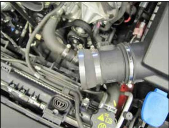
8. Install the provided coupling hose (08618) onto the mass air sensor and secure with the provided hose clamp.
