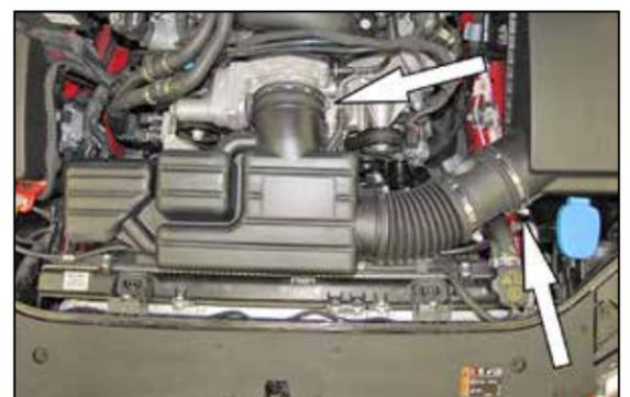
5. Loosen the hose clamps securing the intake plenum to the throttle body and to the mass air sensor then remove the plenum from the vehicle.
