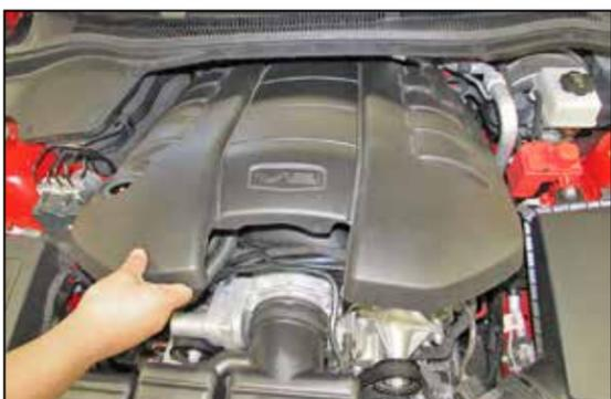
2. Remove the oil fill cap and then remove the decorative engine cover. Reinstall the oil cap to prevent debris from entering the engine.
