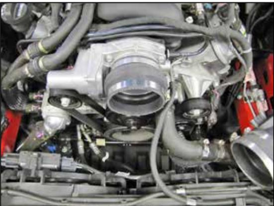
9. Install the provided hump coupler hose (08418) onto the throttle body and secure with the provided hose clamp.
