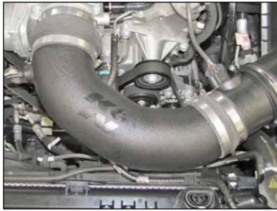
11. Install the K&N® intake tube into the coupling hose at the mass air sensor and then into the hose at the throttle body. Adjust the tube for proper fit and then secure with the provided hose clamps.
