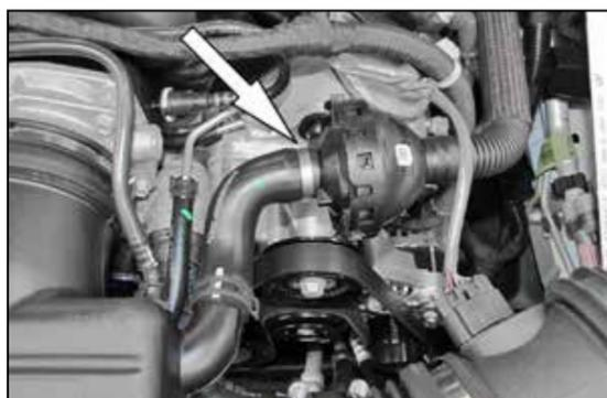
3A. On vehicles equipped with a sound drum, disconnect the sound tube from the drum and cap off the drum with the provided caplug.
