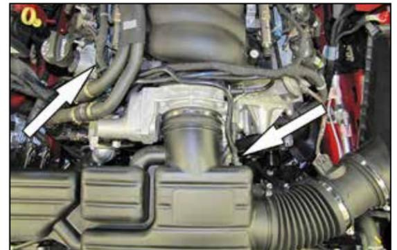
4. Disconnect the crank case vent hose from the intake plenum and valve cover and then remove the hose from the vehicle.
