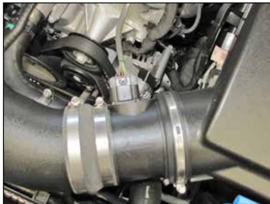
13. Reconnect the mass air sensor electrical connection.
