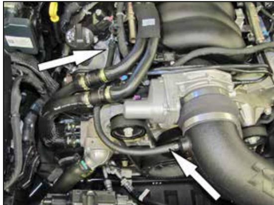
12. Connect the provided crank case vent hose to the fitting installed into the K&N® intake tube and then connect the open end to the port on the valve cover.
