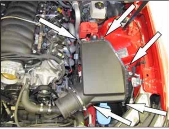
6. Release the five retaining clips and then remove the upper air box assembly.
