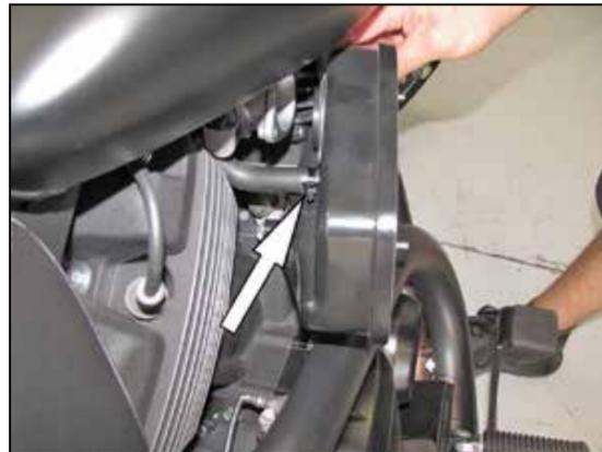
5. Pull the filter back plate away so that the crank case breather hose connection can be accessed. Release the spring clamp and then disconnect the crank case breather and remove the back plate from the vehicle.
