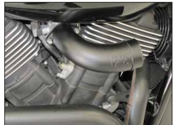
8. Connect the factory crank case breather hose to the fitting installed into the K&N® throttle body adapter tube. Using the factory hardware and gasket, secure the throttle body to the throttle body as shown.
