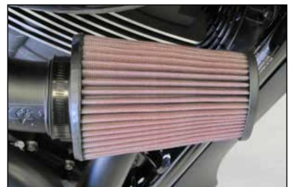
9. Install the K&N® air filter and secure with the provided hose clamp.
