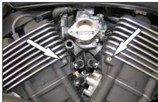
6. Install the two provided button head bolts into the factory air filter back plate mounting locations.
