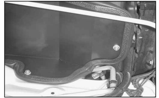
17. Secure the heat shield to the rubber mount studs using the provided hardware.
