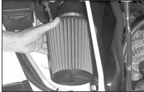
24. Install the K&N air filter element onto the intake tube and tighten with the provided hose clamp.
