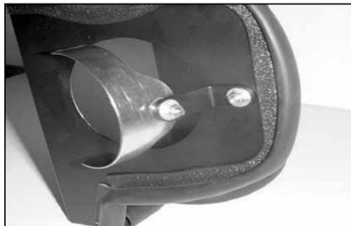
15. Attach the saddle bracket assembly to the heat shield using the provided hardware.
