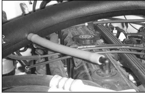
23. Attach the provided vent hose onto the vent fitting of the valve cover and the K&N intake tube.
