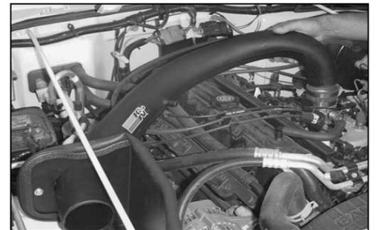
19. Install the K&N® intake tube.
