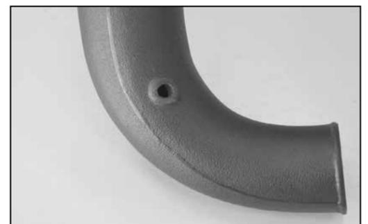
19b. Remove the K&N® intake tube from the vehicle and drill a 3/4" hole at the position marked in step #19a. Install the provided grommet into the hole that was drilled out.
