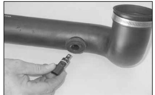
5. On vehicles equipped with a temperature sensor, lift the temperature sensor-locking tab while twisting the sensor counter clockwise to remove the sensor from the intake tube. **NOTE: The temperature sensor is fragile, handle with care.**
