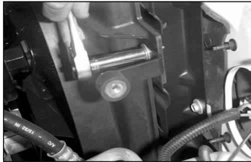
12. Install the "L" bracket using the bolt removed in the previous step.
