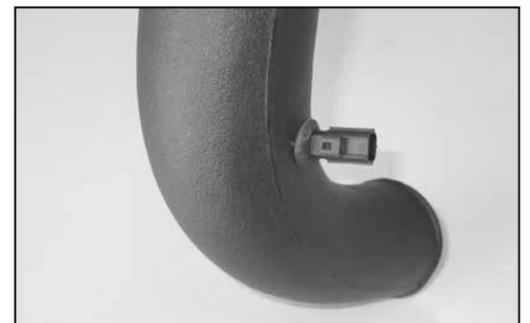
19c. Install the temperature sensor into the grommet as shown.
