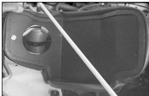
16. Install the heat shield assembly.
