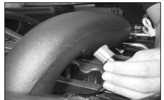
19a. Position the temperature sensor electrical connector next to the K&N® intake tube for the best fit, then mark the location to be drilled.
