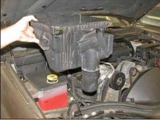
9. Lift the lower airbox and remove it from the vehicle as shown.
