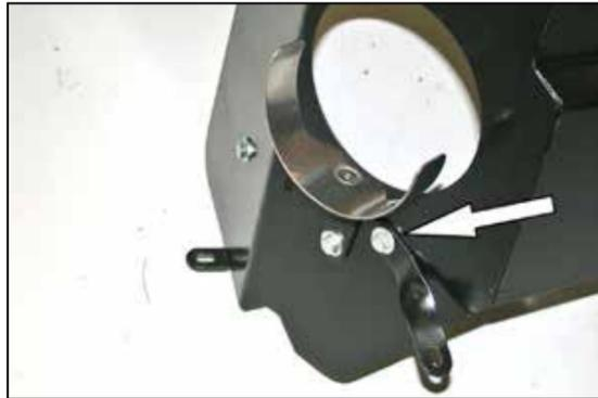
16. Install the twist bracket onto the heat shield as shown using the provided hardware.
