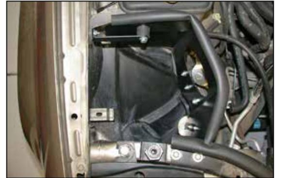
22. Install the heat shield assembly into the vehicle and secure it to the mounting locations with the provided hardware.
