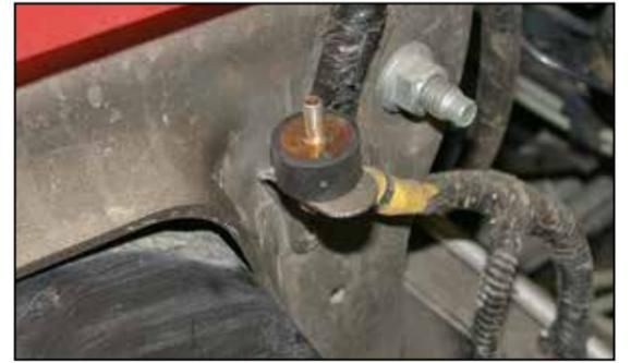
21. Install the 6mm male/male rubber mounted stud onto the upper airbox mount as shown.
