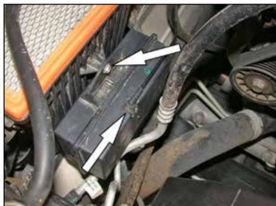
4. Disconnect the vacuum canister hose shown.
