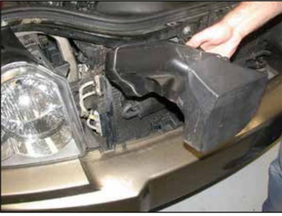
7. Pull the fresh air duct forward to disconnect it from the airbox and then remove it from the vehicle.
