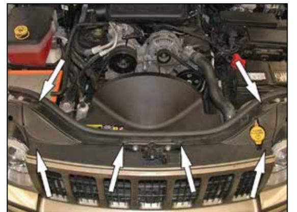
5. Using a small screwdriver, release the center holding pins in the six grill retaining clips shown.
