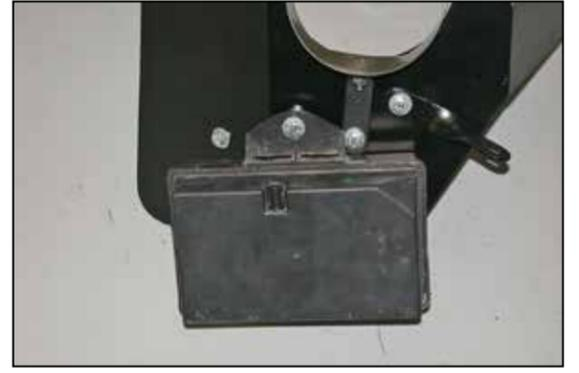
18. Using the provided spacer, install the vacuum reservoir onto the heat shield as shown.
