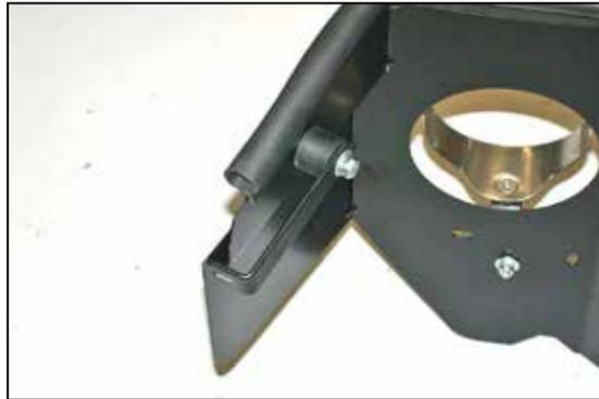
15. Install the bracket/rubber mounted stud assembly onto the heat shield as shown using the provided hardware.
