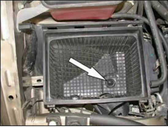
8. Remove the airbox mounting bolt shown.
