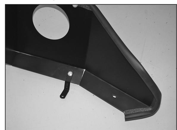
9. Install the "Z" bracket (010120) onto the heat shield with the provided hardware as shown.
