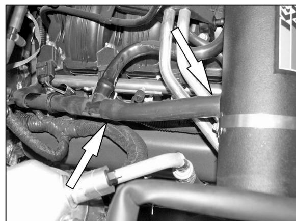
24. Install the provided silicone crank case vent hose onto the factory crank case vent tube and then onto the K&N® intake tube as shown.
