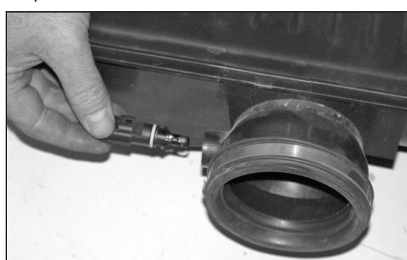
18. Twist the air temperature sensor counter clockwise and remove it from the stock intake plenum.
