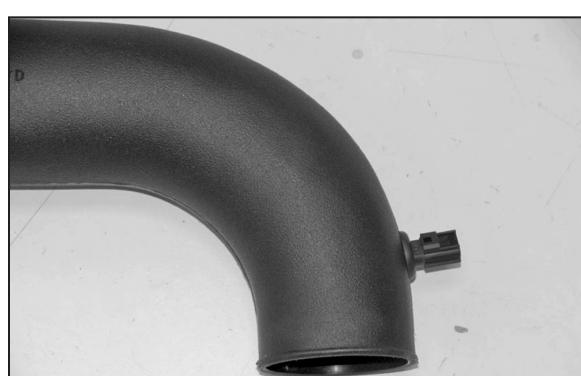
21. Install the sensor into the grommet installed in step #18.
