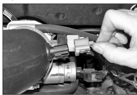
23. Reconnect the air temperature sensor electrical connection as shown.
