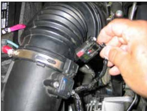
2. Release the red locking clip and then disconnect the mass air sensor electrical connection.
