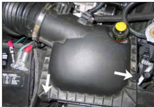
5. Release the two upper air box retaining clips shown.
