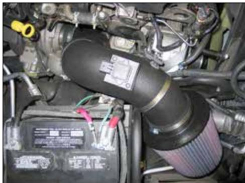
33. Install the intake tube and filter assembly, slide the intake tube into the silicone hose at the turbo and then align with the saddle bracket. Secure the assembly with the provided hose clamps.
