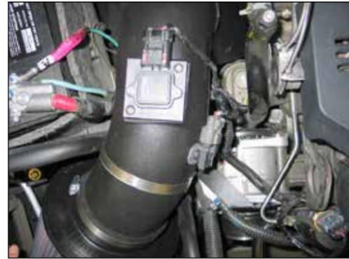
35. Reconnect the mass air sensor and inlet air temperature sensor electrical connections.
