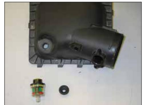
24. On vehicles equipped with filter minder, remove filter minder and grommet from the upper air box as shown.
