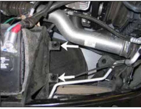
11. Remove the two lower air box mounting grommets from the vehicle.
