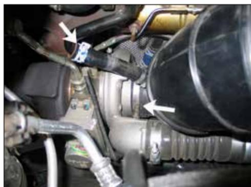
7. Release the tension on the air injection vent hose clamp and the hose clamp which secures the intake tube to the turbo inlet.
