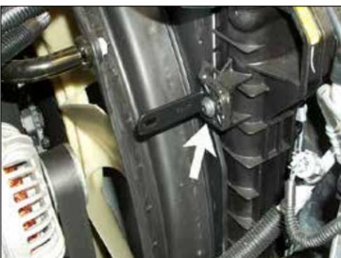
15. Remove the radiator fan shroud bolt. Then install the heat shield mounting bracket (07158) onto the fan shroud using the provided hardware as shown.
