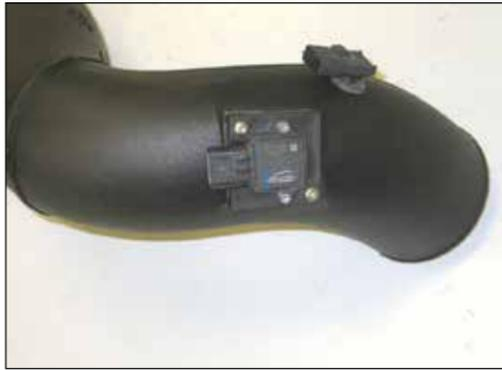
31. Install the mass air sensor assembly into the intake tube and secure with the provided hardware.
