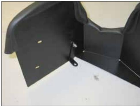
18. Install the heat shield mounting bracket (06723) onto the heat shield using the provided hardware.
