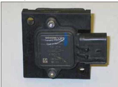
30. Install the mass air sensor into the adapter and secure with the provided hardware.
