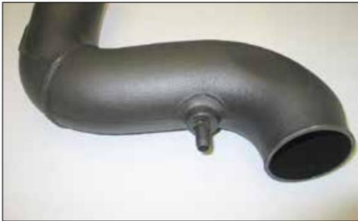
26. Install the provided 1/4"npt fitting into the intake tube as shown.
