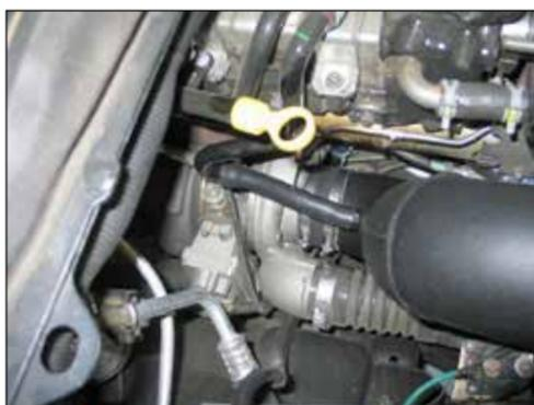
34. Install the provided air injection hose onto the air injection tube and then connect the open end to the 1/4"npt fitting in the K&N® intake tube.
