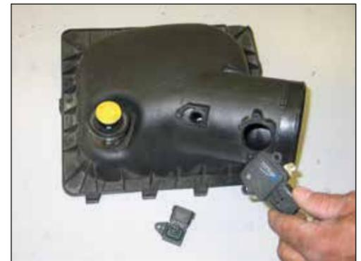
22. Remove the screws which secure the mass air sensor and inlet air temperature sensor and then remove the sensors as shown.
