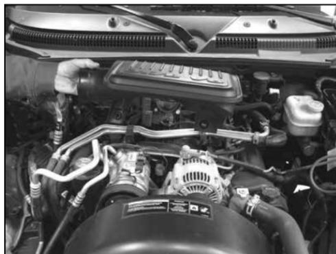
5. Lift to dislodge the intake plenum from its mounting grommets and remove the intake plenum from the vehicle as shown.
