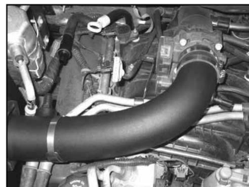
23. Install the K&N® intake tube into the silicone hose on the throttle body and position so the tube aligns with the saddle clamp. Secure the tube with the provided hose clamps.
