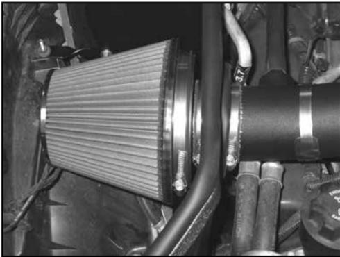
28. Install the air filter assembly onto the K&N® intake tube and secure with the provided hose clamp.
