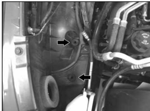
6. Pull the two air box mounting grommets shown from the inner fender.
