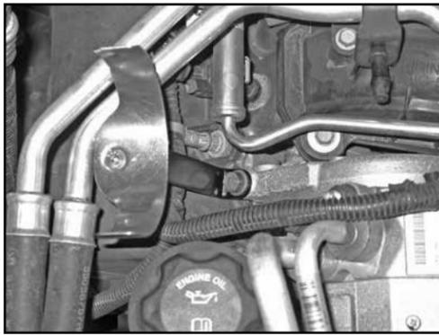
16. Install the tube mounting bracket assembly onto the A/C compressor using the bolt removed in step #14 as shown.
