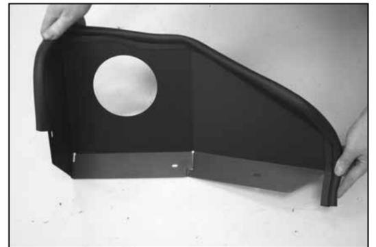
7. Install the provided edge trim onto the heat shield as shown.
