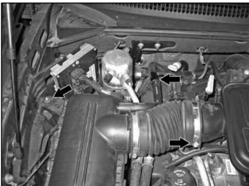
3. Disconnect the stock intake tube from the intake plenum. Lift to remove to remove the air box assembly from the vehicle as shown.
