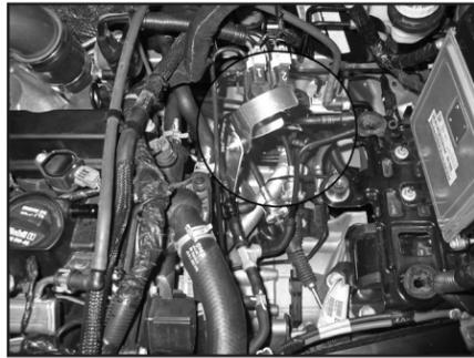
17. Secure the intake tube mounting bracket to the driver's side of the tab on the transmission using the provided hardware.
