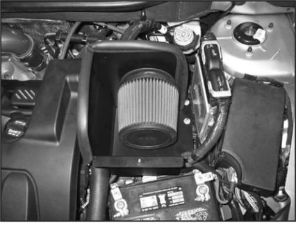
28. Install the K&N® air filter onto the intake tube and secure with the provided hose clamp.
