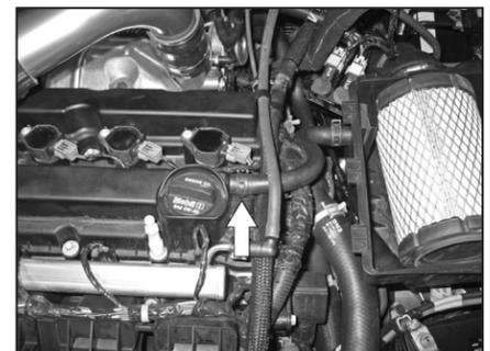
8. Release the spring clamp that secures the crank case breather hose to the valve cover. Then disconnect the crank case breather hose.
