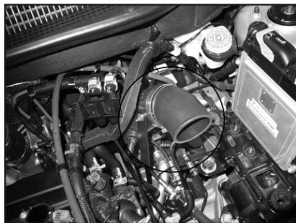
19. Install the K&N® intake tube into the silicone hose at the turbo inlet and align with the mounting bracket, then secure with the provided hose clamps.
