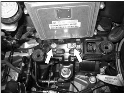
14. Remove the two ECU mounting nuts shown.
