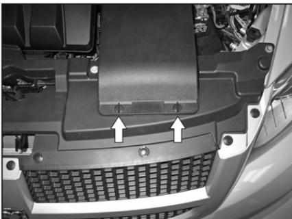
2. Unlock the two fresh air retaining clips by turning a 1/4 turn counter clockwise.
