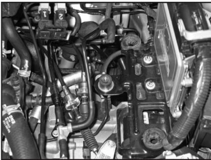
13. Install the rubber mounted stud into the center air box mounting location as shown.
