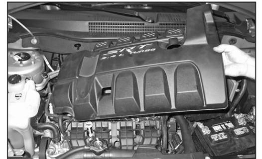
7. Lift up the engine cover to dislodge it from the mounting studs and then remove the engine cover from the vehicle.
