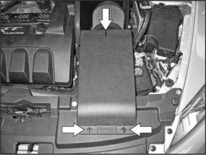
29. Install the fresh air intake duct onto the core support and heat shield, and then secure with the factory ¼ turn clips and hardware provided.
