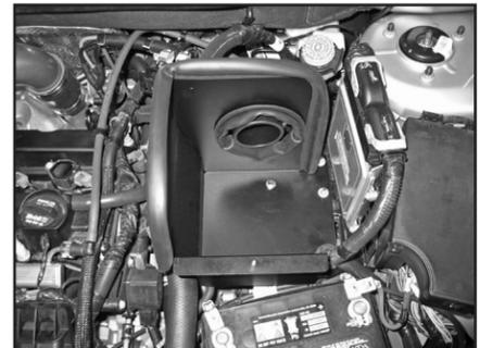
24. Install the heat shield onto the rubber mounted stud installed during step #13 and onto the ECU mounting studs. Then secure the heat shield with the factory ECU mounting bolts and hardware provided.
