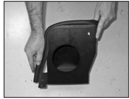
22. Install the provided edge trim onto the heat shield as shown.
