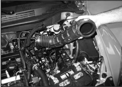
11. Loosen the hose clamp that secures the intake hose to the turbo inlet and then remove the intake tube from the vehicle.
