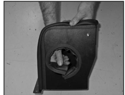
23. Install the provided edge trim into the hole of the heat shield as shown.
