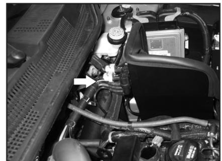
25. Secure the vacuum solenoids to the stud on the back of the heat shield using the provided hardware.
