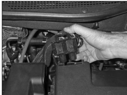
4. Release the clip which holds the vacuum switches to the upper air box and then unhook the vacuum switches from the air box.
