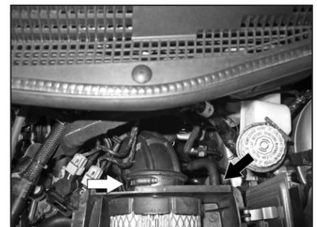
9. Loosen the hose clamp that secures the factory intake hose to the air box. Then unhook both the intake hose and vent hose from the air box.
