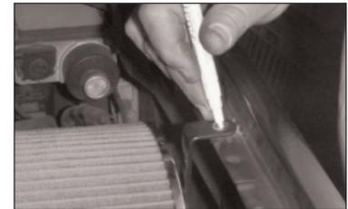
14. Line up the "L" bracket with the fender and mark hole.
