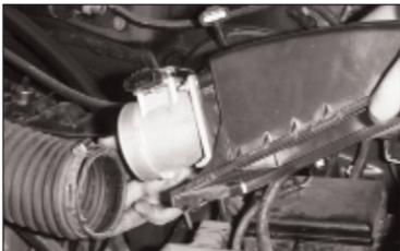
4. Release the two over center clips and remove the airbox top assembly.
