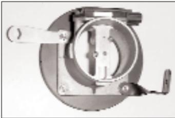
9. Assemble the mass air sensor, mass air adapter, twist bracket and air temperature sensor bracket as shown in the above illustration.
