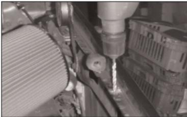
17. Remove the air filter assembly, then drill a hole at the locations marked in step 14 and 15.
