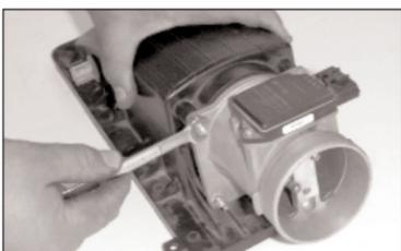
6. Detach the air inlet duct from the airbox base and remove the airbox base.
