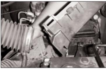
7. Loosen and remove the four nuts that secure the mass air sensor to the airbox top. Remove the mass air sensor from the airbox top.
