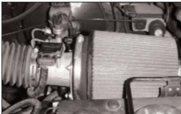
24. Reconnect the mass air sensor and air temperature sensor electrical connection.
