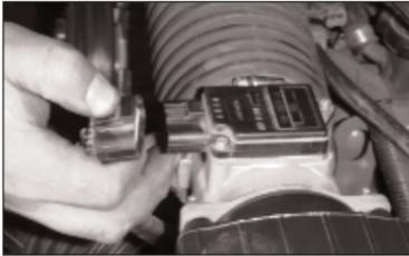
2. Disconnect the vehicle's mass air sensor and air temperature sensor electrical connections.
