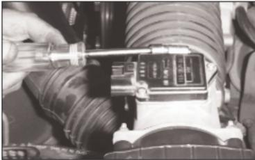
3. Loosen the hose clamp on the intake tube at the mass air sensor.
