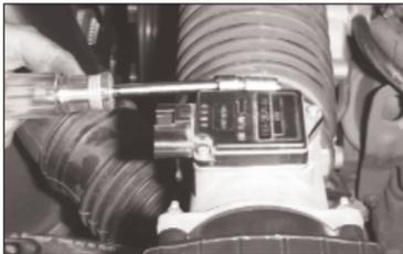
21. Twist the air temperature sensor a 1/4 turn and remove it from the airbox top.
