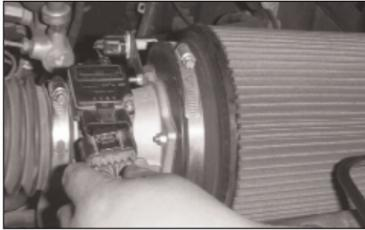
23. Reconnect the mass air sensor and air temperature sensor electrical connection.
