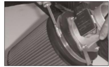
12. Attach the air filter assembly onto the mass air adapter and secure with hose clamp.
