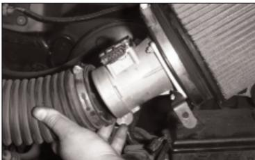
19. Attach the intake tube to the mass air sensor and tighten the hose clamp.
