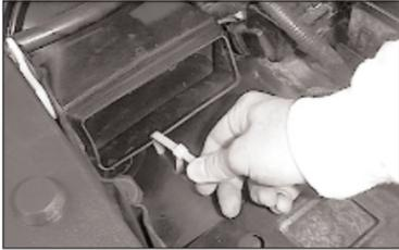
18. Drill a hole through the air inlet duct and the inner fender well, then secure using the zip tie provided.
