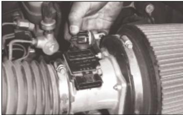
22. Install the air temperature sensor into the air temp sensor bracket and twist a 1/4 turn.
