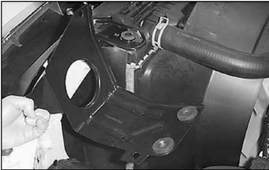
10. Remove the air cleaner mounting bracket.
