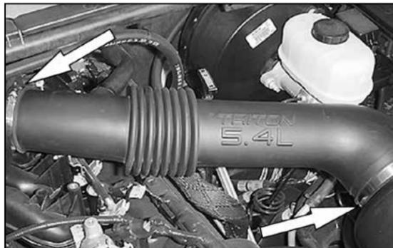
6. Loosen the hose clamps on the stock intake tube at the air cleaner and throttle body.
