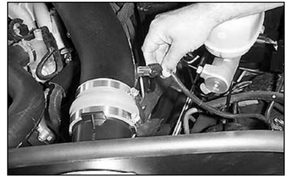
36. On models equipped with an external air temperature sensor, reconnect the air temperature sensor electrical connection and relocate the wiring harness retaining clip to front hole in the inner fender apron.
