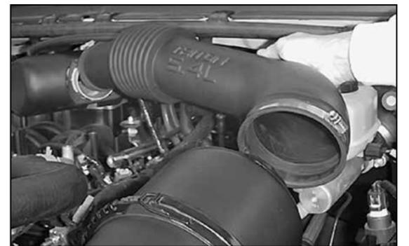
7. Remove the stock intake tube.
