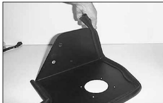
19. Install the trim seal onto the heat shield as shown.
