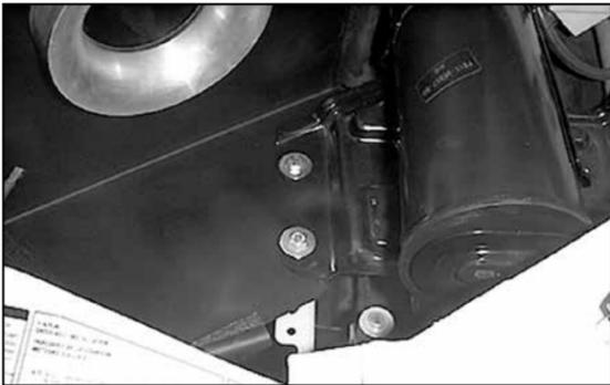
27. Install the hardware to retain the heat shield.
