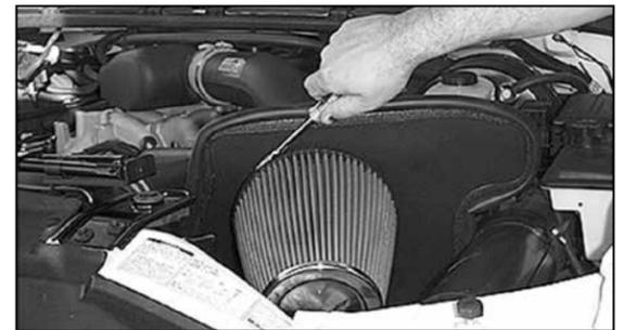
37. Install the air filter and tighten hose clamp.
