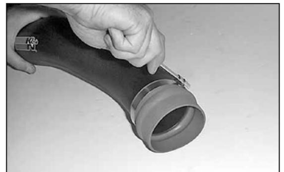
25. Install the hump hose onto the intake tube and tighten hose clamp.
