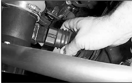
33. Reconnect the primary mass air sensor electrical connection.
