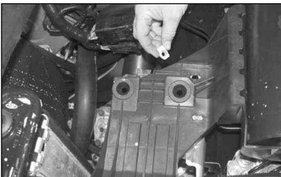
13a. On 2004 and later vehicles remove the clip nuts from under the air box-evap bracket as shown.
