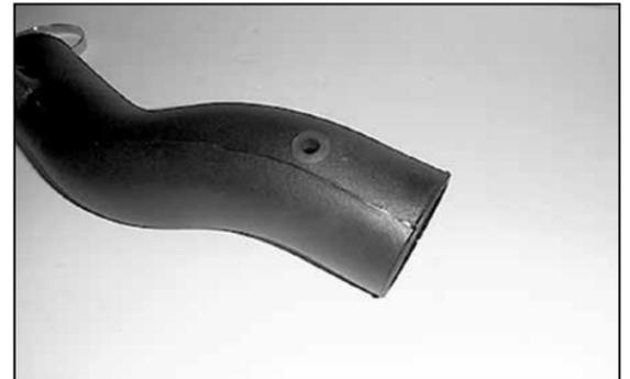
23. On models equipped with an external air temperature sensor, insert the grommet into the hole drilled in the K&N® intake tube.
