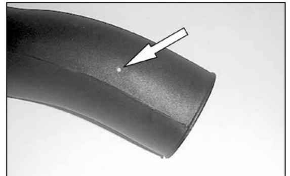
22. On models equipped with an external air temperature sensor, drill out the drill point in the K&N® intake tube using a 11/16" drill bit.
