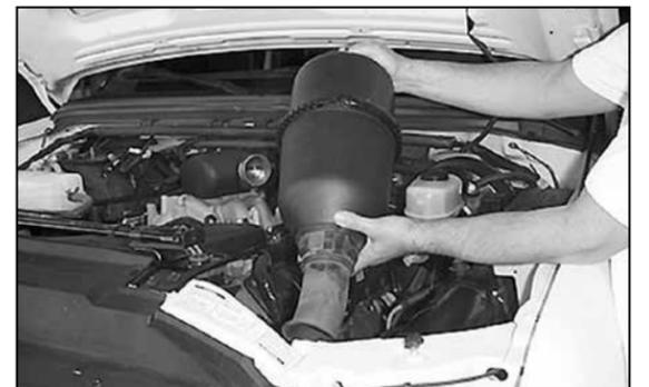
8. Pull upward firmly and remove the air cleaner.
