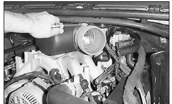
24. Install the stepped hose onto the throttle body and tighten hose clamp.
