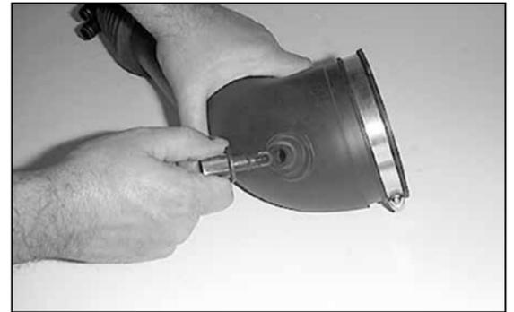
21. On models equipped with an external air temperature sensor, remove the air temperature sensor from the stock intake tube.
