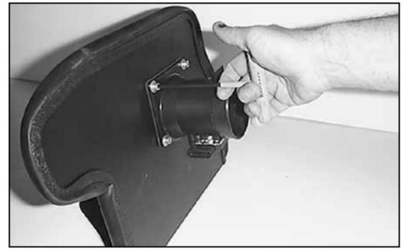
20. Assemble mass air sensor, heat shield and adapter using the gaskets and hardware provided.
