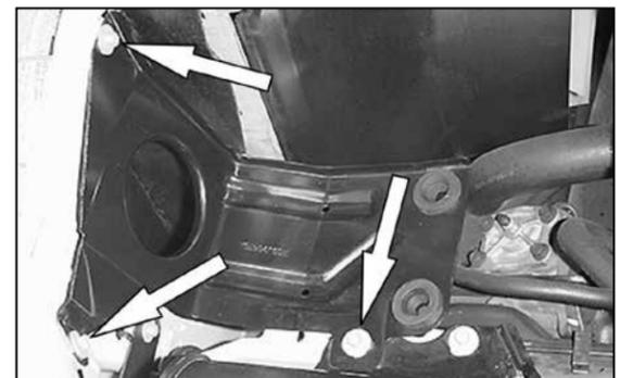
9. Loosen and remove the three bolts that retain the air cleaner mounting bracket.
