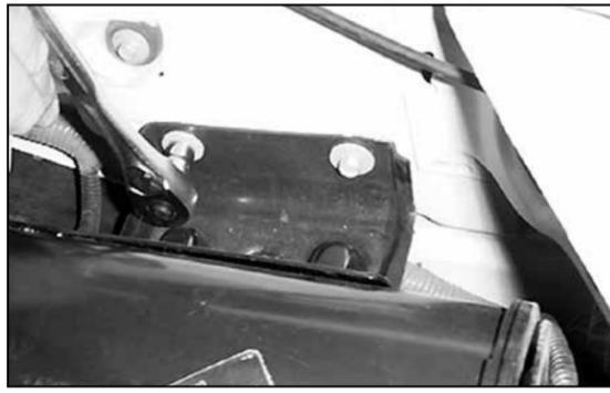
30. Tighten the two bolts that retain the evaporative canister mounting bracket to the inner fender.
