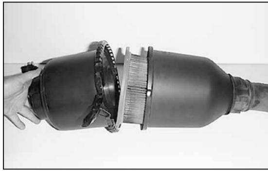
14. Disassemble the air cleaner assembly.
