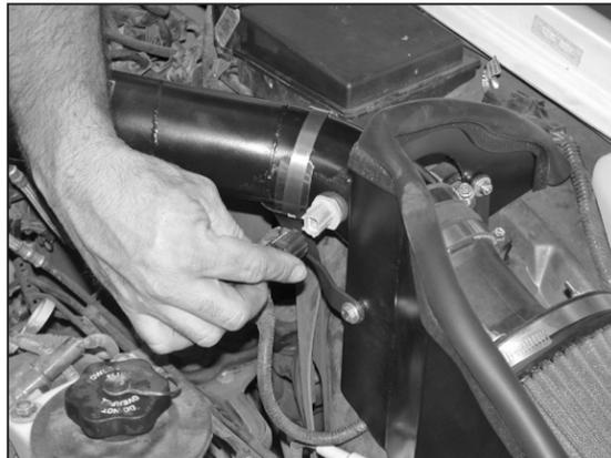
28. On vehicles with external temp sensor, install the temp sensor onto the intake tube then re-connect the electrical connection.
