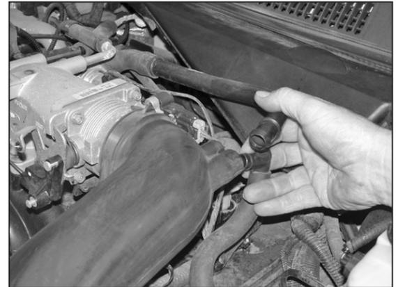
5. Disconnect the crankcase vent and idle air hoses as shown.
