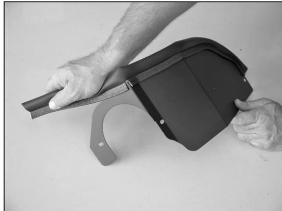
14. Install edge trim onto heat shield as shown. Trim if needed.
