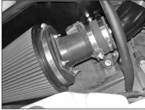
27. Install the mass air assembly onto the intake tube and adjust for best fit before tightening hose clamps.
