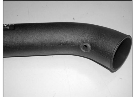
18. On vehicles that come with external temp sensor drill out the drill point with a 3/4 drill, then install the provided grommet as shown.
