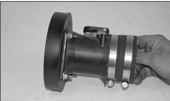
24. Install the silicone hose (08690) onto the mass air sensor with provided hose clamps as shown.
