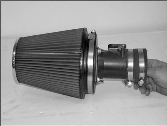
25. Install the air filter onto the mass air assembly as shown.
