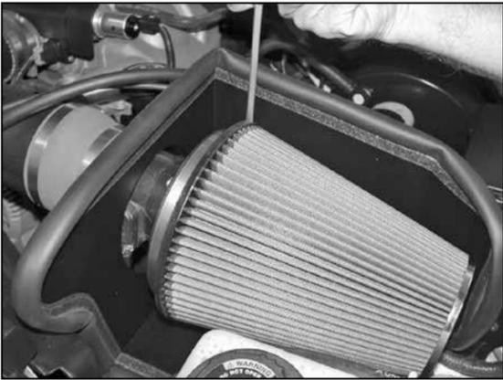
30. Install the K&N® air filter onto the mass air sensor and secure it with the provided hose clamp.
