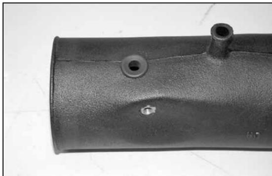
20. Install the provided grommet into the new intake tube as shown.
