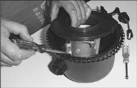
11. Using a flat blade screwdriver, push in and release the four clips that retain the mass air sensor retaining plate.
