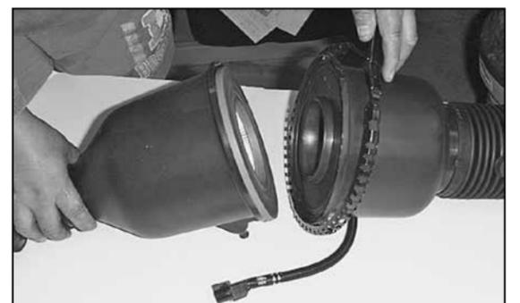
9. Open the air cleaner assembly and isolate the mass air sensor assembly.
