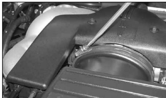
5. Loosen hose clamp at the throttle body.
