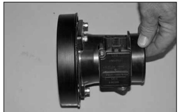
26. Attach the mass air adapter to the mass air sensor using the gasket and provided hardware as shown.
