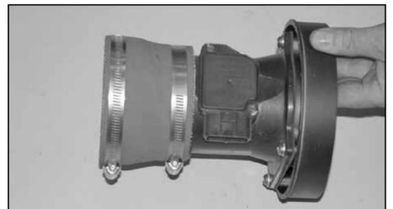
27. Install the silicone hose (08050) onto the mass air assembly with provided hose clamp as shown.
