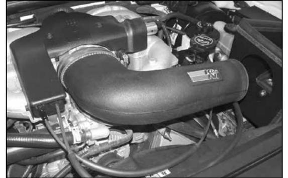
23. Install the new K&N® intake tube onto the silicone hose.
