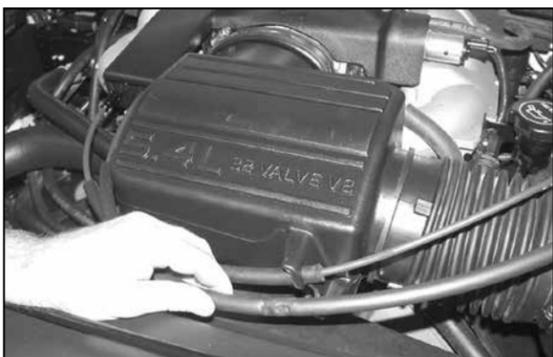
2. Unhook and remove speed control cable and throttle cable from the stock intake tube.
