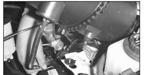
7. Disconnect the secondary mass air sensor electrical connection.
