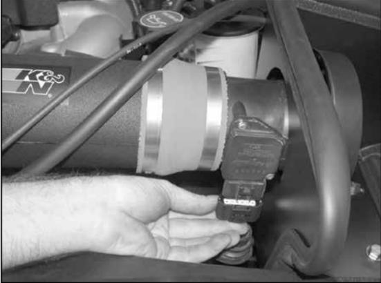
29. Reconnect the primary and secondary mass air electrical connection.
