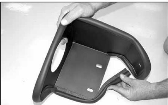
14. Install edge trim onto heat shield as shown. Trim if needed.
