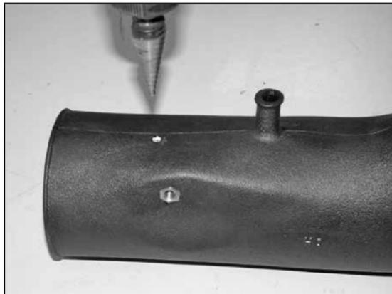
19. On vehicles equipped with an air temp sensor. Drill a 5/8" hole at the drill point indicated on the K&N® intake tube.
