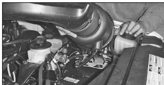
6. Detach the stock intake tube from the throttle body and lift up on the air cleaner assembly to release it from its retaining grommets.
