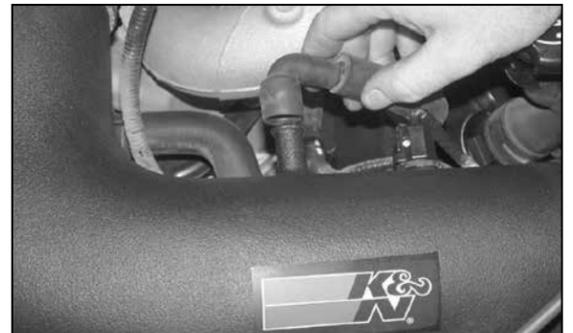
25. Install the air temp sensor into the K&N® intake tube, reconnect the air temp electrical connection and install crank case vent onto the vent port.
