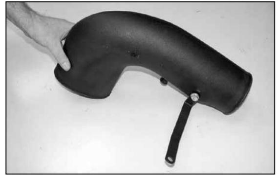
22. Install the provided bracket (07169) onto the K&N® intake tube with hardware provided.
