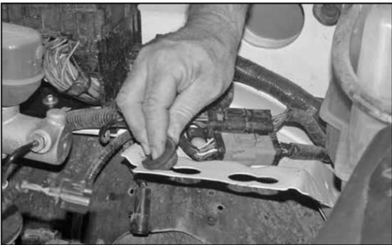
13. Remove the two air box mounting grommets from vehicle as shown.
