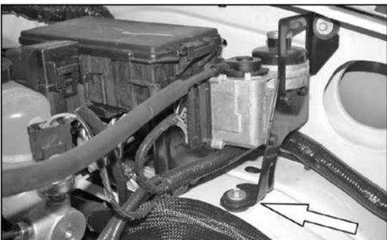
15. Remove the 6mm bolt that retains the cruise control onto vehicle.
