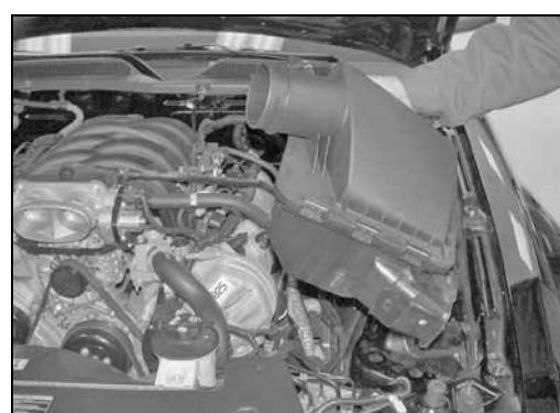
6. Remove the air box assembly as shown.
