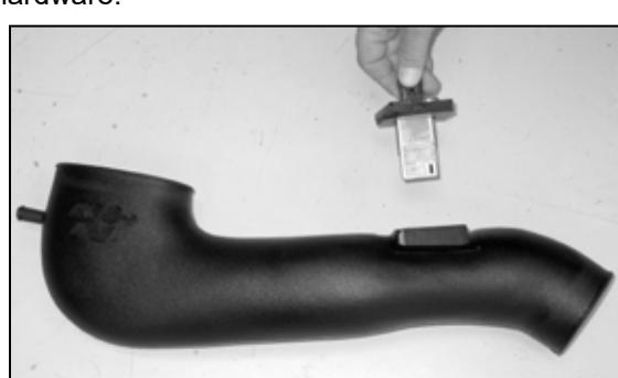
17b. Install the mass air sensor assembly into the K&N® intake tube and secure with the provided hardware.
