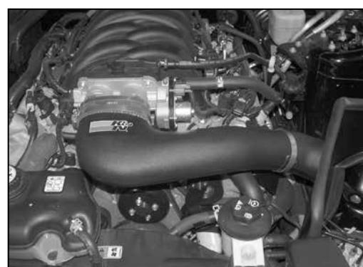
19. Install the K&N® intake tube into the silicone hose at the throttle body and onto the saddle bracket assembly then secure with the provided hose clamps as shown.
