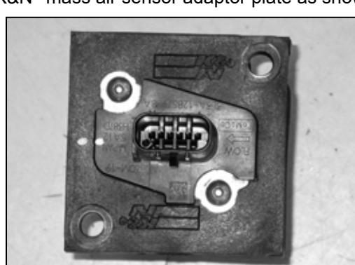
17a. Install the mass air sensor into the K&N® mass air sensor adaptor and secure with the provided hardware.
