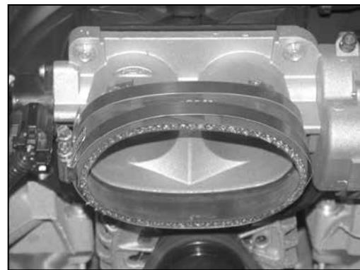
18. Install the silicone hose (08541) onto the throttle body with the provided hose clamps as shown.
