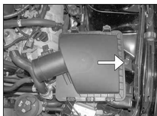
5. Remove the air box mounting bolt shown.
