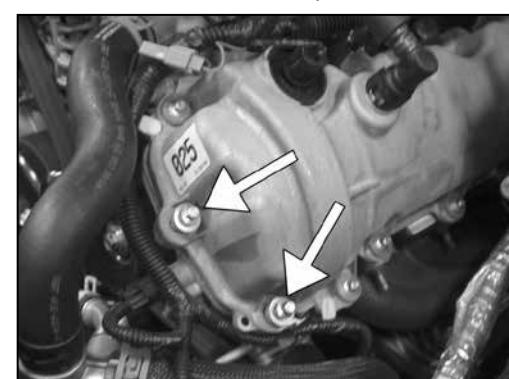
8. Remove the two valve cover bolts shown.
