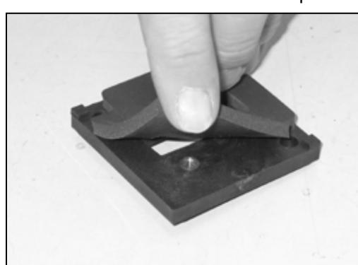
17. Install the provided gasket to the back of the K&N® mass air sensor adaptor plate as shown.
