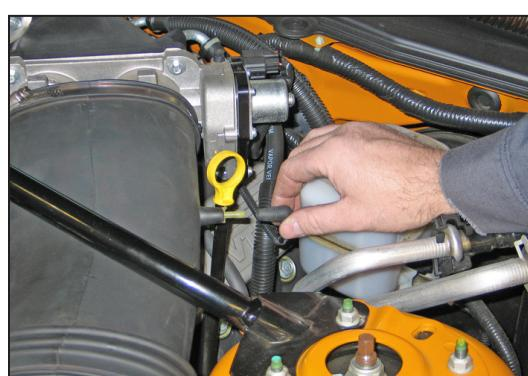
4. Disconnect the vacuum vent line as shown.
