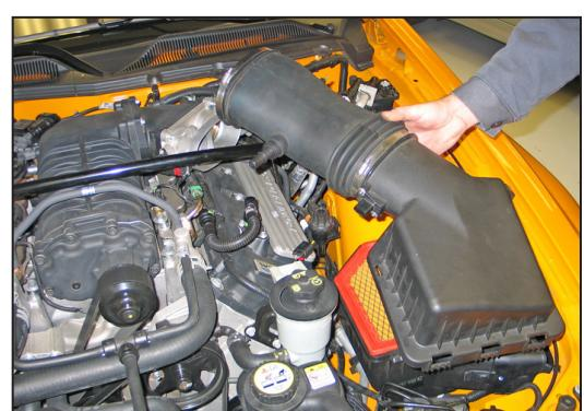
7. Remove the intake tube and airbox lid from the vehicle.
