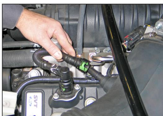
3. Rotate the green locking tab and then disconnect the crankcase vent hose from the intake tube.
