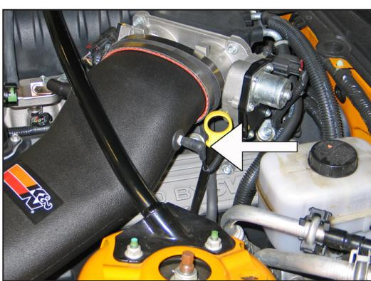
25. Connect the vacuum vent line onto the  $\frac{1}{4}$ " hose mender that was inserted in the K&N® intake tube during step #13.
