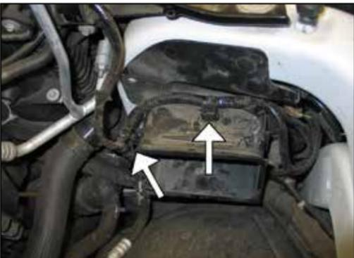
14. Unhook the wiring harness from the fresh air intake duct.
