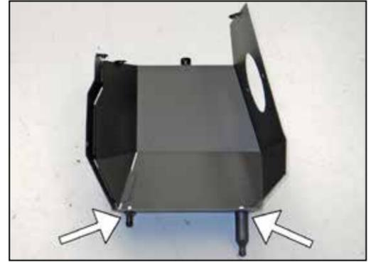
20. Install the two heat shield stand-offs onto the heat shield as shown using the provided hardware.
