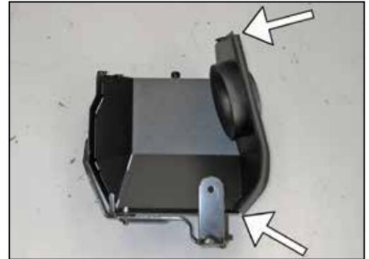
23. Install the provided edge trim onto the heat shield as shown.
