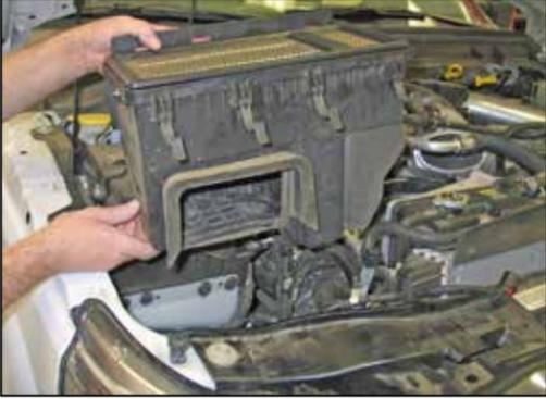
11. Remove the lower air box from the vehicle.
