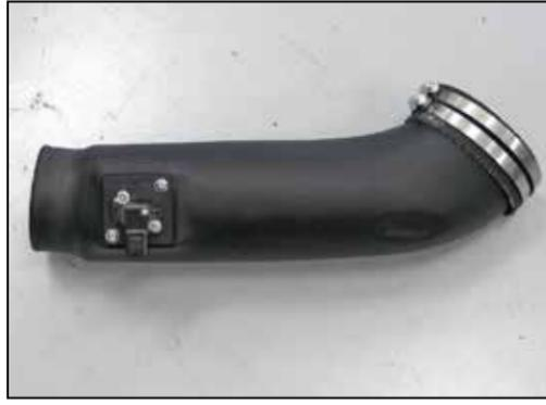
30. Install the provided silicone hose (08540) all the way onto the K&N® intake tube so the end of the tube is exposed.
