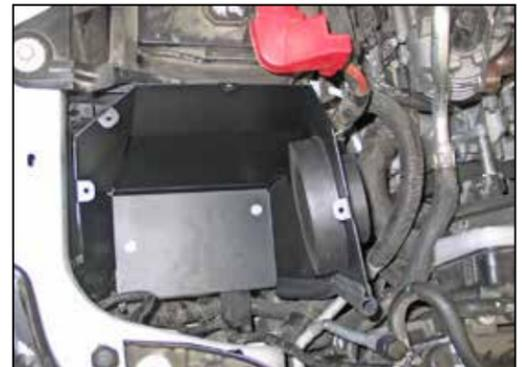
24. Set the heat shield assembly into position and secure with the factory mounting hardware from step #12.
