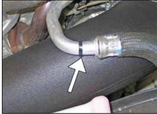
32. Secure the coolant pipe to the insert of the K&N® intake tube with the provided mounting tie wrap.
