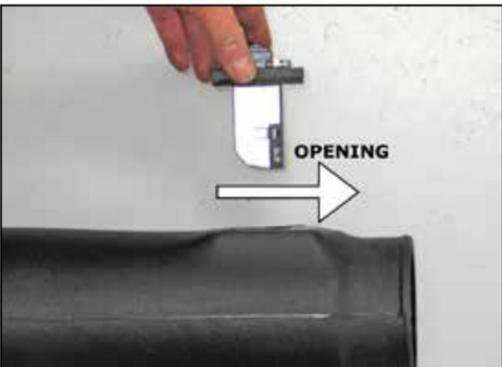
29. Install the mass air sensor assembly into the K&N® intake tube as shown and secure with the provided hardware.
