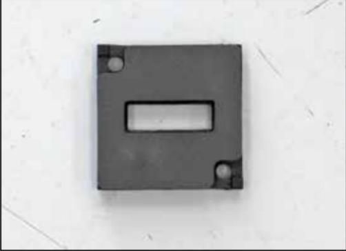
26. Attach the provided gasket onto the mass air sensor adapter as shown.
