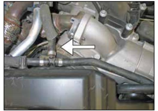
8. Loosen the hose clamp that secures the intake tube to the engine inlet.
