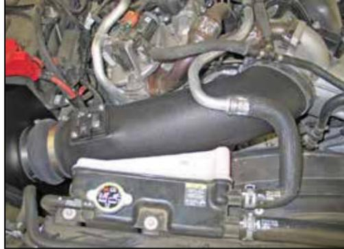
31. Install the intake tube into the silicone hose attached to the filter adapter and align the tube with the factory intake. Slide the silicone hose onto the factory intake and then secure the tube with the hose clamps.
