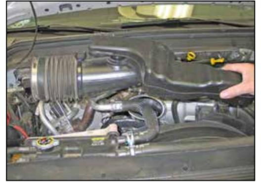
9. Remove the intake tube from the vehicle.
