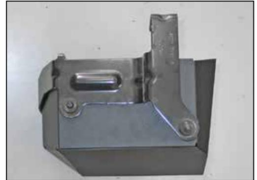
22. Install the factory air box mounting bracket onto the heat shield as shown so that the mount stand-offs installed in step #20 snap into the factory mounting grommets.
