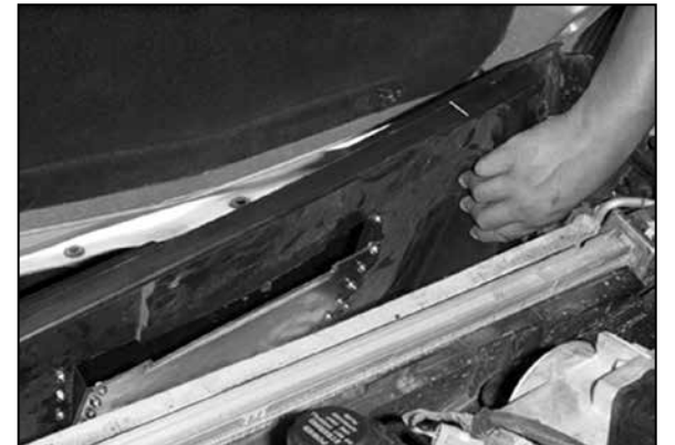
43. Reinstall the lower radiator cover.
