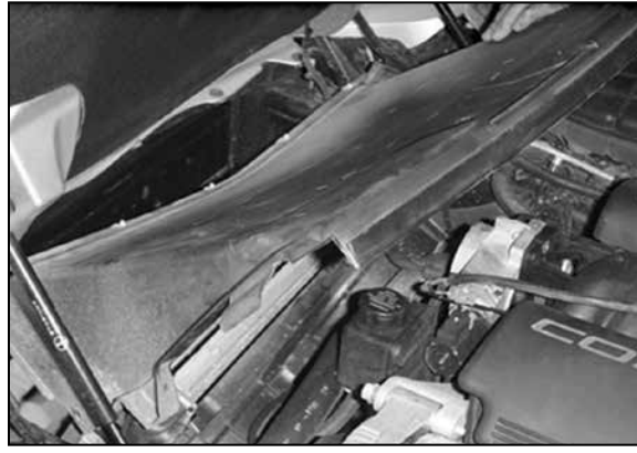
34. Remove the lower radiator cover.
