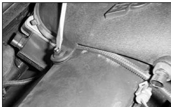
4. Release the push clips that retain the stock intake tube to the upper radiator cover.
