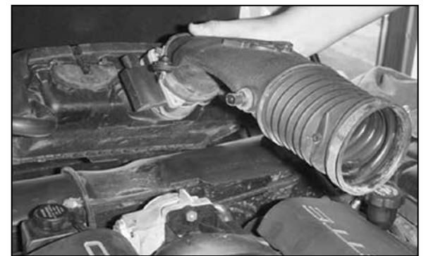
7. Detach the intake hose from the throttle body and remove the entire air intake assembly. NOTE: K&N Engineering, Inc., recommends that customers do not discard factory air intake.
