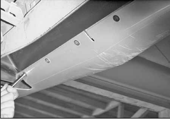
30. Loosen and remove the five bolts that mount the lower radiator cover to the bumper cover on the underside of the car.
