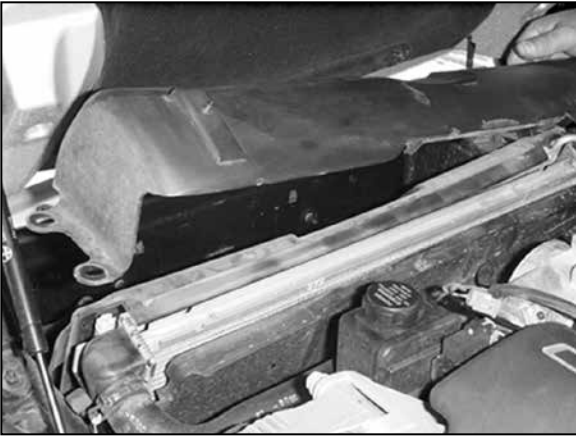
29. Remove the upper radiator cover.
