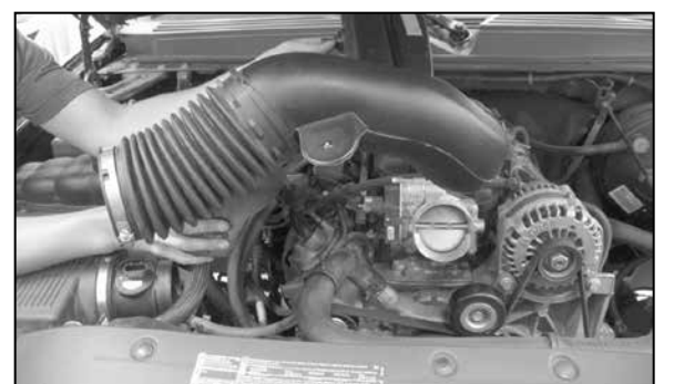
6. Loosen the hose clamps, which secure stock intake tube to the throttle body and mass air sensor and then remove the intake tube from the vehicle.
