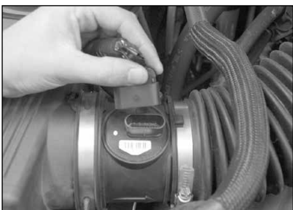
2. Disconnect the mass air sensor electrical connection.
