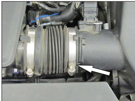
3. Loosen the hose clamp securing the factory intake hose to the air filter housing.
