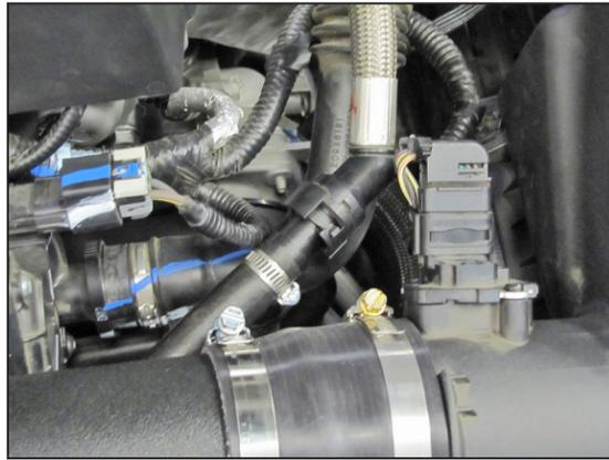
14. Connect the factory crank case vent fitting into the K&N® quick connect fitting as shown.
