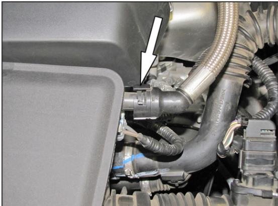
2. Unlock the crank case vent hose locking ring and then disconnect the crank case vent hose from the intake plenum.
