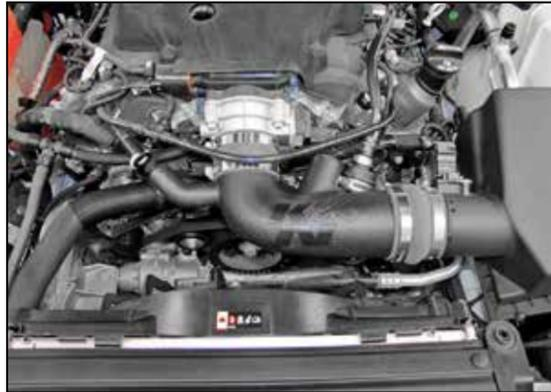
14. Install the K&N® intake tube into the coupling hose at the air box and then into the coupler at the throttle body, adjust the tube for best fit and then secure with the provided hose clamps.
