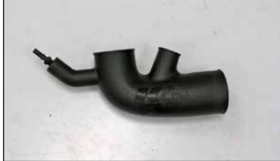
13. Install the provided quick disconnect NPT fitting into the K&N® intake tube as shown.
