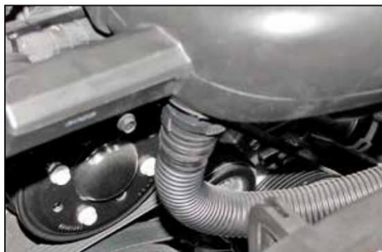
4. On vehicles equipped with an engine sound tube, release the sound tube quick disconnect fitting and disconnect the sound tube from the factory intake tube.
