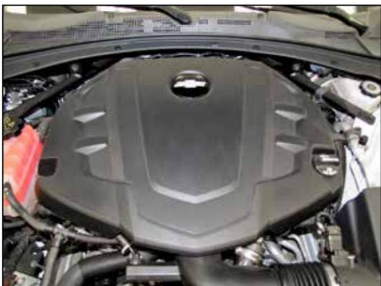
2. Remove the bolt that secures the decorative engine cover, remove the oil cap and then remove the decorative engine cover. Reinstall the oil cap.
