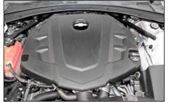
17. Reinstall the decorative engine cover and secure with the factory bolt and oil cap.
