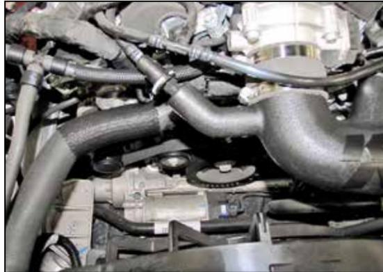
15. Connect the factory EVAP hose quick connector to the quick connector installed into the K&N® intake tube.
