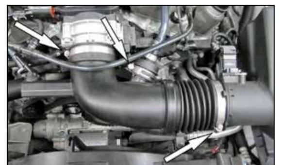
5. Loosen the three hose clamps that secure the intake tube and crank case vent tube and remove the intake tube from the vehicle.
