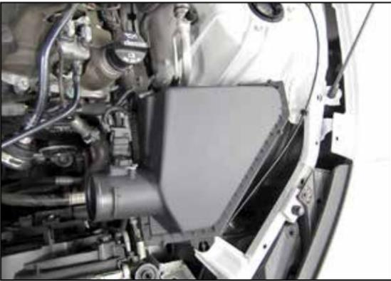
9. Loosen the screws that secure the upper air filter housing.
