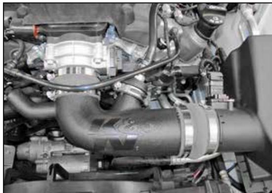
16. Connect the crank case fitting onto the K&N® intake tube and secure with the provided hose clamp.
