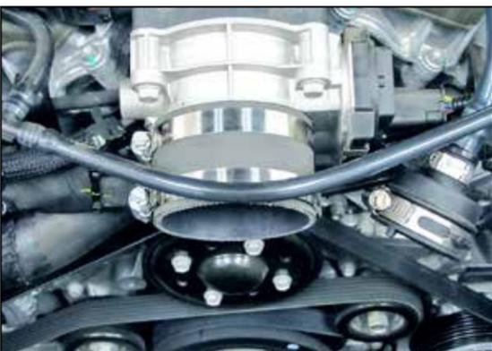
11. Install the provided coupling hose (084031) onto the throttle body and secure with the provided hose clamp.
