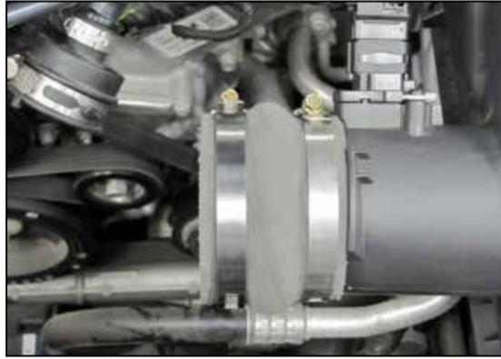
12. Install the provided hump coupler hose (08171) onto the Mass air sensor outlet and secure with the provided hose clamp.
