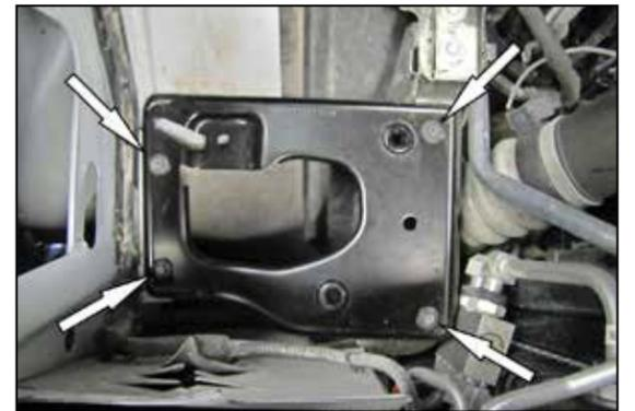
5. Remove the four bolts that secure air filter mounting tray and then remove the tray from the vehicle. Three of the factory bolts will be reused in a later step.
