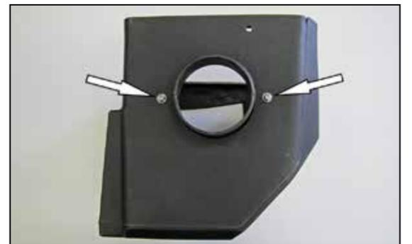
6. Install the filter adapter into the K&N® air filter housing and secure with the provided hardware.
