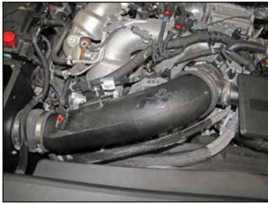
12. Install the K&N® intake tube assembly into the coupler at the filter adapter and then into the factory turbo inlet coupler. Adjust the tube for best fit and then secure with the hose clamps.
