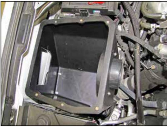
7. Install the K&N® air filter housing into the vehicle and secure it to the factory housing mounting plate fastener location with the hardware removed in step 5.
