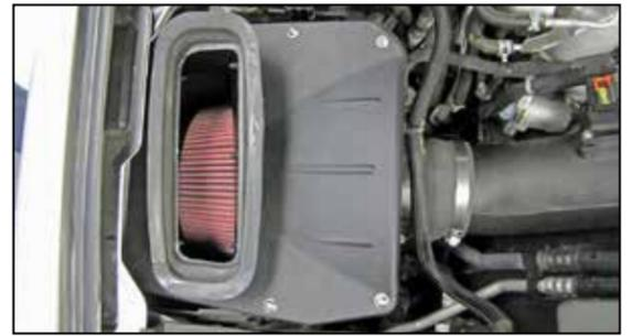
17. Install the K&N® air filter housing lid onto the filter housing and secure with the provided hardware.
