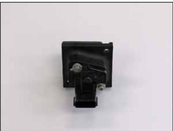
10. Remove the mass air sensor from the factory air filter housing and then install it into the K&N® adapter and secure with the provided hardware.
