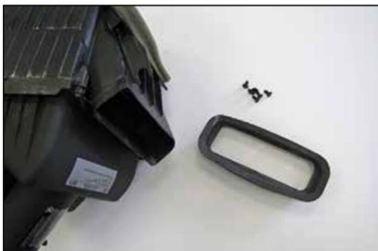
15. Remove the fresh air bellows from the factory air filter housing lid.
