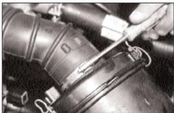
3. Loosen the hose clamp and disconnect the intake tube from the air cleaner assembly. **NOTE:** Remove the factory hose clamp as it will not be reused.
