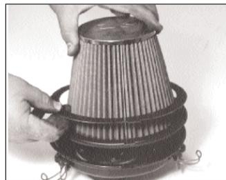
12. Install the Filtercharger Element along with the provided retaining ring onto the upper portion of the air cleaner assembly, then secure into place using the three over center clips as shown above.
