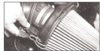
15. Re-connect the mass-air sensor electrical connection.
