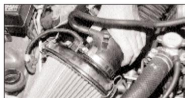
13a. On the 1990 models, install the filtercharger assembly into the stock intake hose with the locating tab in the 12 o'clock position. Secure the intake hose to the saddle with the hose clamp provided as shown above.
