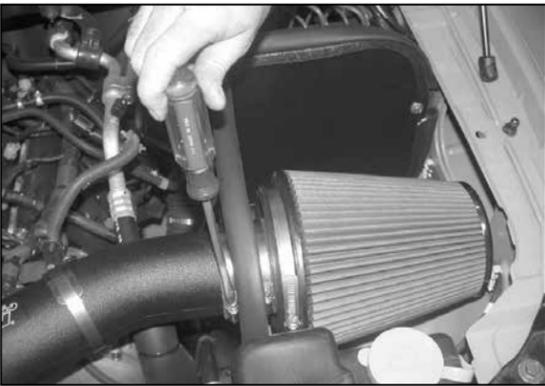
30. Install the K&N® air filter assembly onto the K&N® intake tube as shown; secure with the provided hose clamp.
