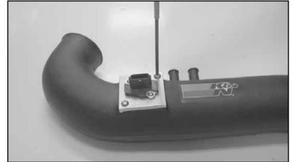
23. Secure the mass air sensor assembly onto the K&N® intake tube with the provided hardware.
