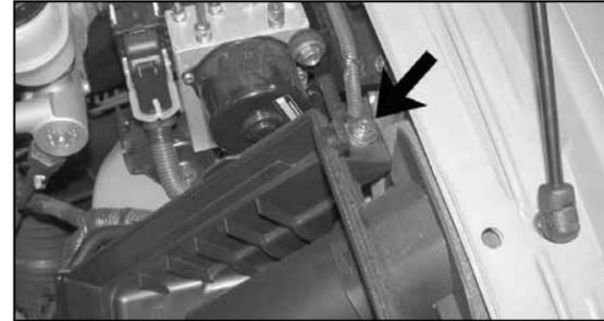
7. Remove the air box mounting bolt with a 10mm socket.
