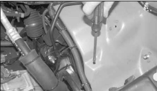
13. Using a screw driver, push the center of the plastic inner fender retaining clip through, then remove the clip from the inner fender.
