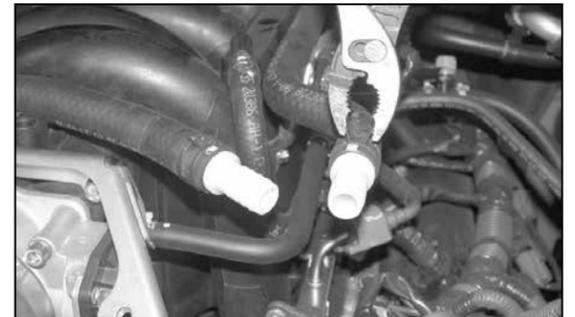
26. Install the provided hose mender into the two crank case vent hoses and secure the existing spring clamps as shown.
