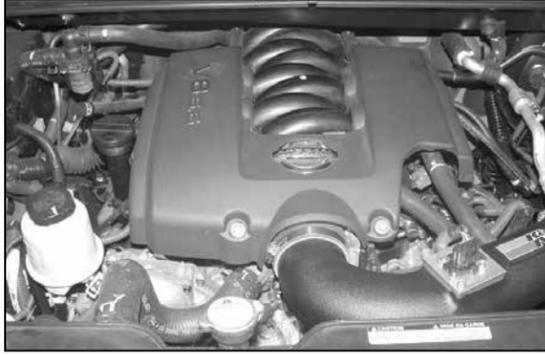
32. Re-install the throttle body cover as shown.
