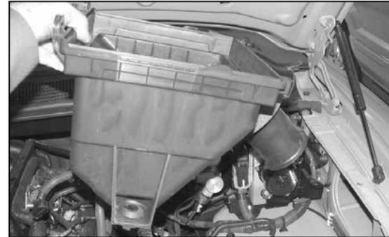
8. Pull firmly up on the air box to release it from the mounting studs, then remove the air box from the vehicle.
