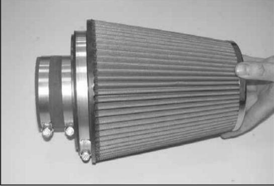
29. Install the filter adapter assembly into the K&N® air filter.
