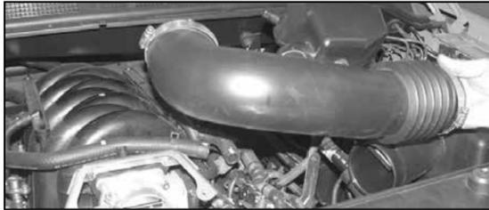
5. Loosen the hose clamps at the throttle body and air box, then remove the intake tube from the vehicle.
