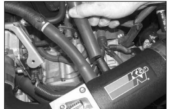
27. Install the provided silicone hose onto the hose mender, then install the hoses onto the intake tube as shown.
