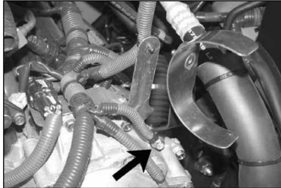
17. Install the saddle bracket assembly and ground wire removed in step #16 with the provided hardware as shown.
