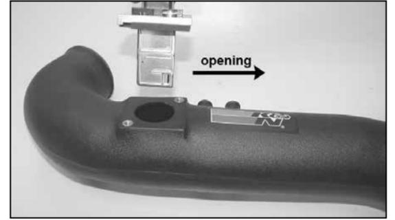
22. Install the mass air sensor assembly into the intake tube with the opening of the sensor pointing towards the air filter end of the tube as shown.
