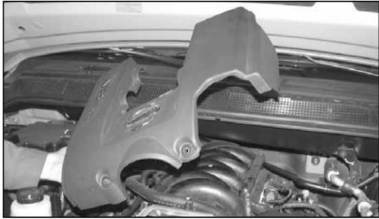
2. Remove the two bolts that secure the throttle body cover, then remove the throttle body cover.
