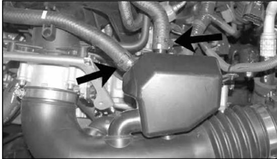
4. Remove the two vent lines from the air intake resonator as shown.
