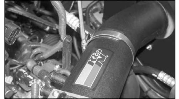
25. Secure the K&N® intake tube to the saddle bracket with the provided hose clamp. Also tighten the hose clamp at the throttle body.
