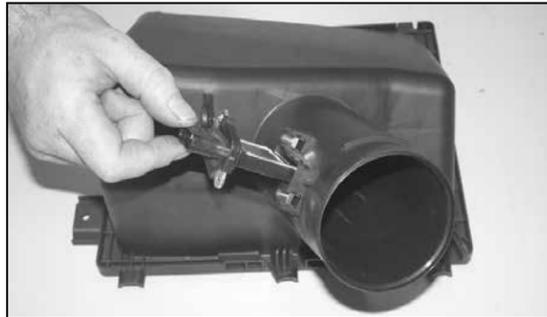
19. Remove the two screws that secure the mass air sensor to the air box lid, then remove the mass air sensor as shown.
