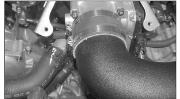
24. Install the K&N® intake tube onto the throttle body and align with the saddle bracket.
