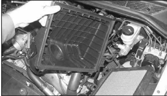
6. Release the two air box lid retainer clips that secure the air box lid to the air box, then remove the air box lid and air filter.
