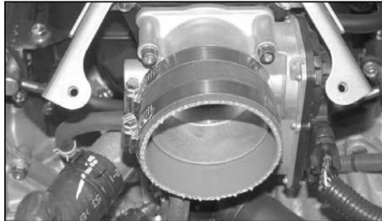
18. Install the provided silicone hose (08690) onto the throttle body with the provided hose clamps as shown.
