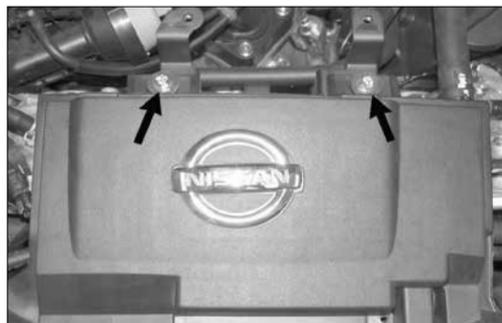
5. Remove the two bolts shown which secure the stock intake tube to the engine.
