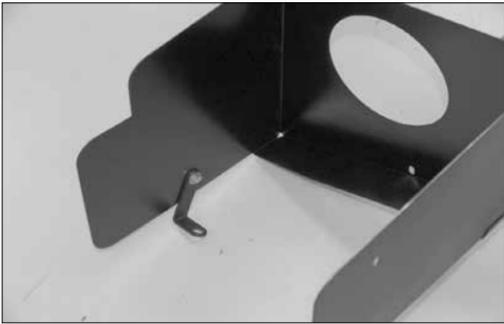
12. Install the "L" bracket (070632) onto the heat shield as shown with the provided hardware.
