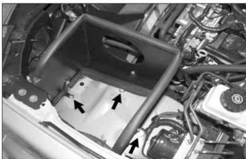
19. Install the heat shield assembly into the vehicle and secure with the provided hardware to the air box mounting locations.
