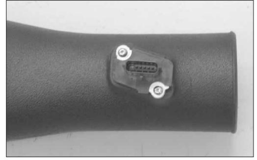
22. Install the mass air sensor into the K&N® intake tube and secure with the hardware provided.
