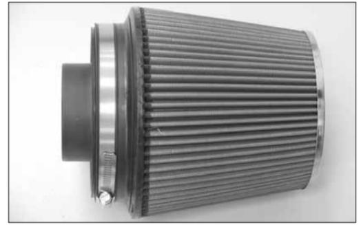
25. Install the filter adapter into the air filter as shown and secure with the provided hose clamp.
