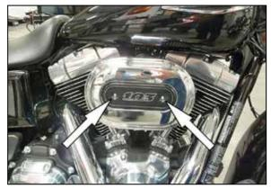
2. Remove the two screws that attach the number plate.
