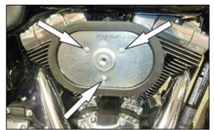
4. Remove the three air filter retaining bolts shown.
