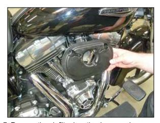
7. Remove the air filter breather base as shown. NOTE: K&N Engineering, INC. recommends that customers do not discard the factory air intake components.
