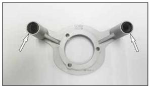
8. Install two of the o rings provided onto the back side of the K&N® back plate as shown.
