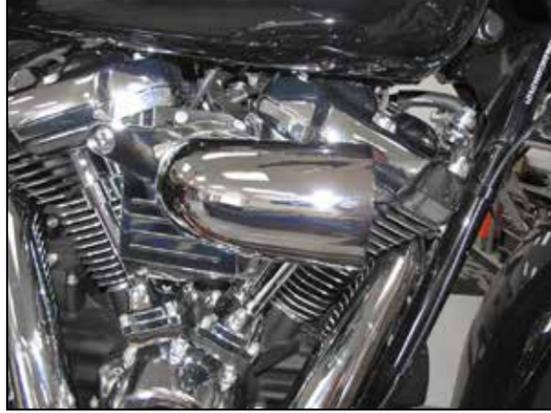
10. Install the intake tube onto the base plate.
