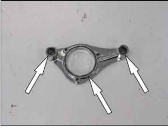
7. Install two of the breather O-rings and the throttle body O-ring into the base plate as shown.
