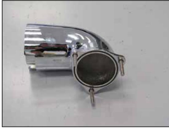
9. Install the provided O-ring and tube mounting bolts into the intake tube as shown.
