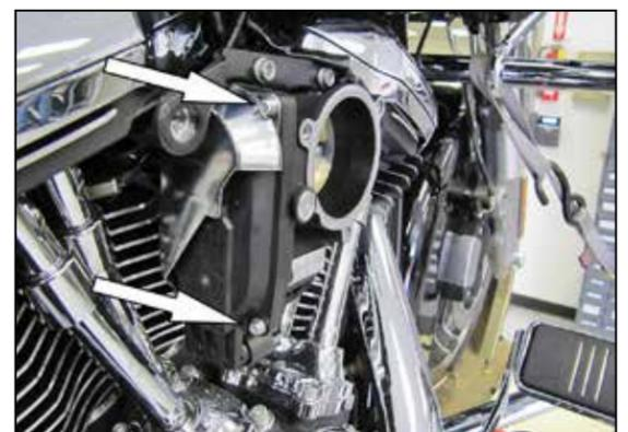
5. Remove the two servo cover bolts shown.
