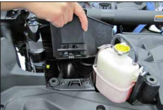
9. Lift and remove the clutch filter.
