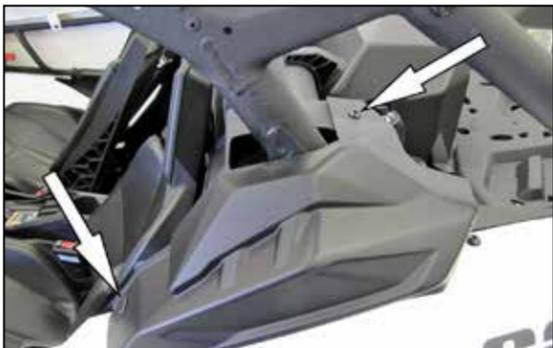
2. Remove the two fasteners securing the corner cap and then remove the corner cap from the vehicle.
