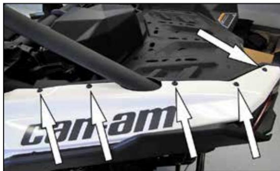
3. Remove the five fasteners and clip nuts securing the top of the fender.
