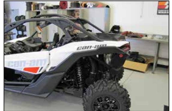
34. Reinstall the fender and corner cover and secure with the factory hardware and clips.
