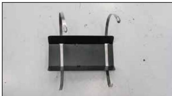
17. Install the two large hose clamps into the air filter housing mounting bracket as shown.
