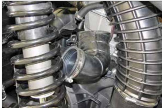
14. Loosen the hose clamp securing the clutch intake hose and disconnect the hose and set aside for access to the air filter assembly.
