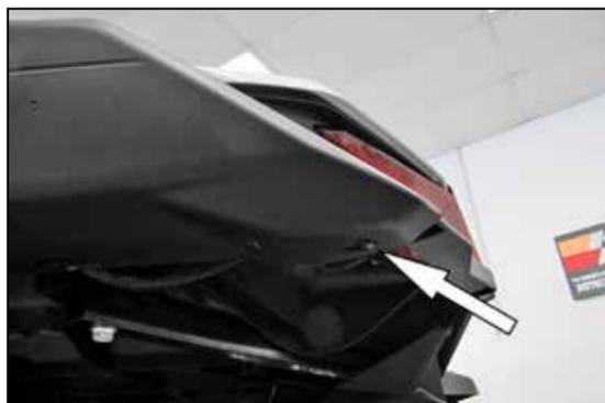
4. Remove the fastener on the bottom side near the tail light.
