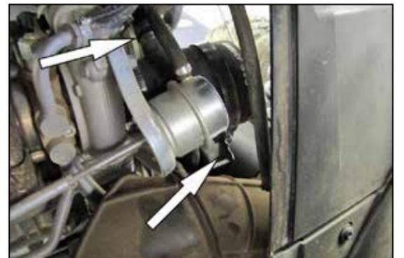
20. Install the K&N® intake hose assembly (084103) onto the turbo, rotate the hose so that the crank case vent hose aligns with the fitting installed into the K&N® hose. Install the crank case vent hose and secure with the factory hose clamp. Connect the vacuum hose to the fitting installed into the K&N® intake hose. It may be necessary to use the extra hose mender and hose provided due to manufacturer changes.
