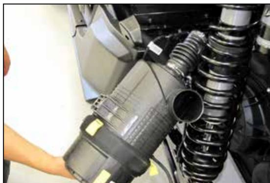
16. Remove the air filter housing assembly from the vehicle.
