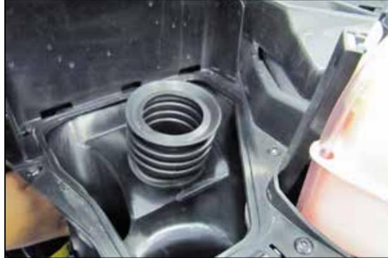
13. Remove the intake flex hose from the plenum.
