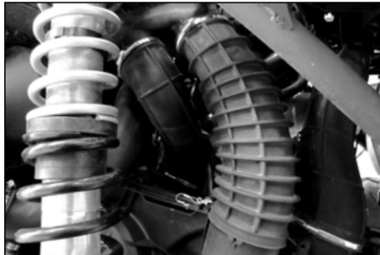
30. Reinstall the clutch fresh air intake hose and secure with the factory hose clamp. **NOTE: On models that have a resonator in the factory clutch hose, install the clutch has provided using the factory clamps.**
