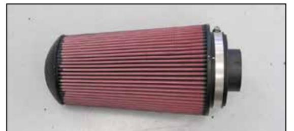
21. Install the filter adapter into the K&N® air filter and secure with the provided hose clamp.
