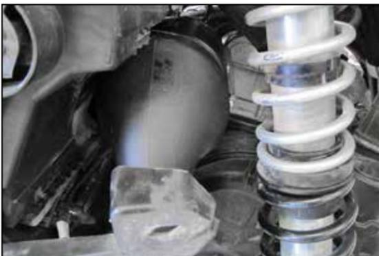
24. Install the air filter housing assembly onto the bracket and into the coupling hose at the turbo. Secure the housing with the hose clamps attached to the mounting bracket. Do not completely tighten at this time.
