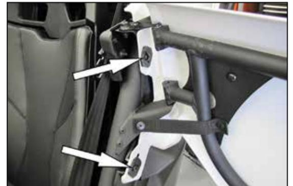
6. Open the door and remove the two fasteners securing the front of the fender.
