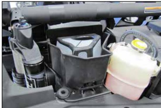
32. Reinstall the clutch filter assembly.
