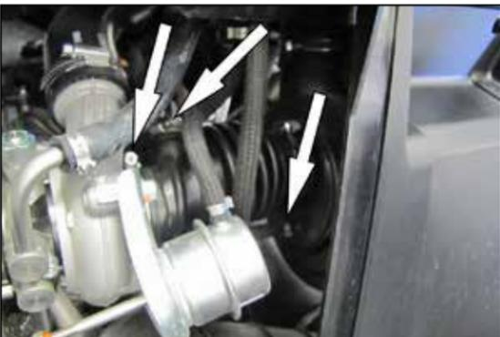
11. Loosen the hose clamp that secures the crank case vent hose to the intake hose and then disconnect the crank case vent hose. Cut the clamp that secures the vacuum hose to the air filter housing and then disconnect the vacuum hose. Loosen the hose clamp that secures the intake hose to the turbo inlet.
