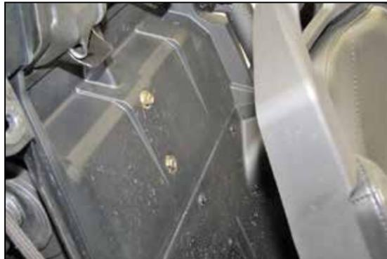
15. Remove the two bolts located behind the seat that secure the air filter housing to the firewall.
