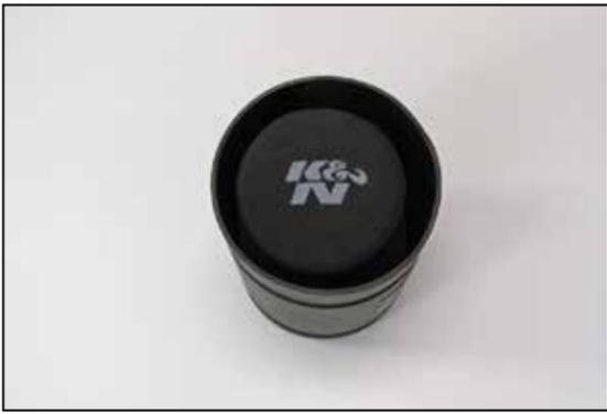
22. Install the K&N® air filter into the K&N® air filter housing and secure with the provided hardware.
