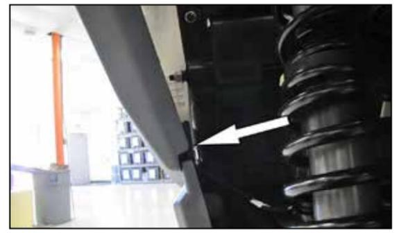
5. Remove the fastener securing the back side of the fender to the lower fender.
