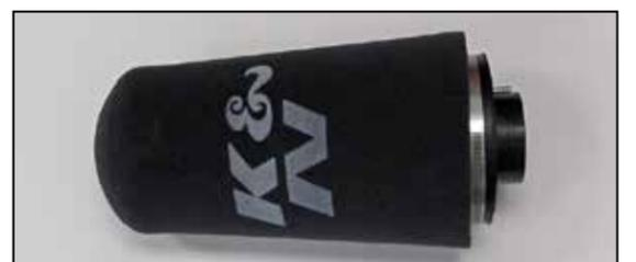
21a. Install the pre-wrap onto the K&N® air filter.
