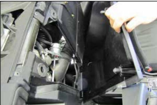
10. Remove the turbo access panel from the firewall between the seats.
