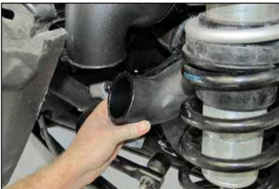
26. Feed the fresh air intake tube up into its location.
