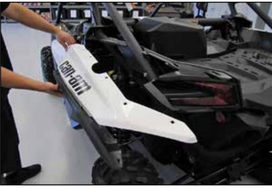
7. Remove the fender partially and then unhook the tail lamp harness from the fender and then completely remove the fender from the vehicle.
