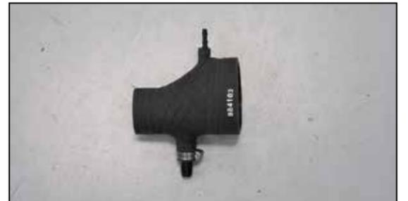
19. Install the two provided vent fittings into the K&N® intake hose (084103) and secure the large fitting with the provided hose clamp.
