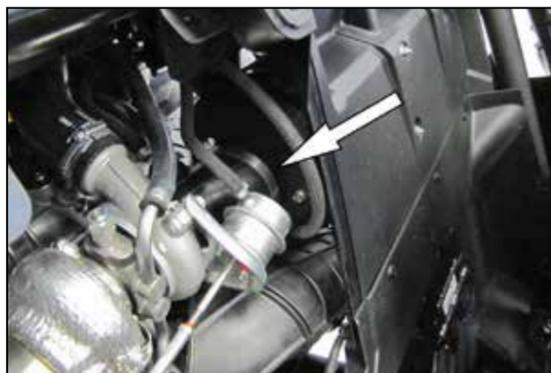
31. Be sure the turbo inlet hose is fully seated onto the filter adapter and then secure the hose with the provided hose clamp. Reinstall the access panel.
