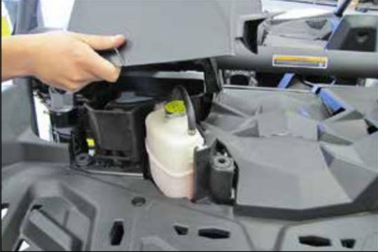
8. Lift and remove the air intake cover.
