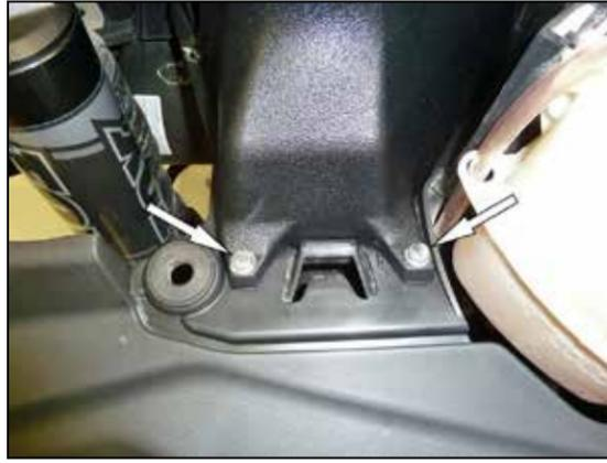
10. Install the K&N® fresh air system and secure with the provided hardware.
