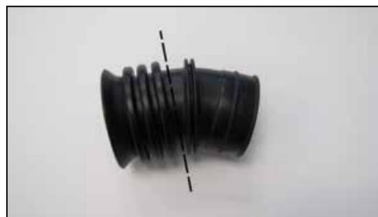
4. If intake kit 57-1141 is not previously installed, remove the factory bellows from the vehicle and trim it where indicated and then reinstall the bellows.
