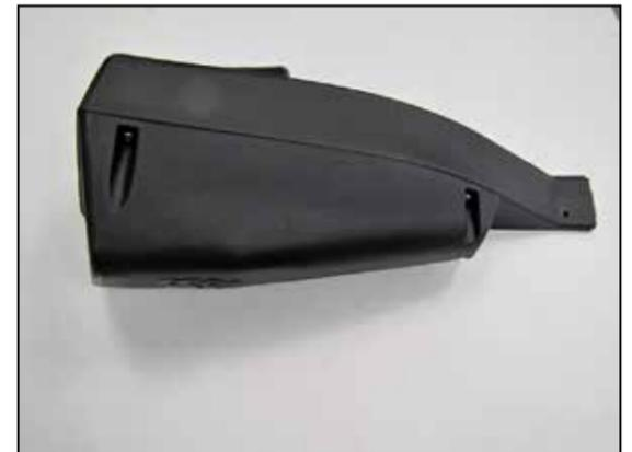
4. Assemble the left K&N® prefilter/scoop by placing the prefilter onto the housing and then installing the scoop onto the housings and secure with the provided hardware.
