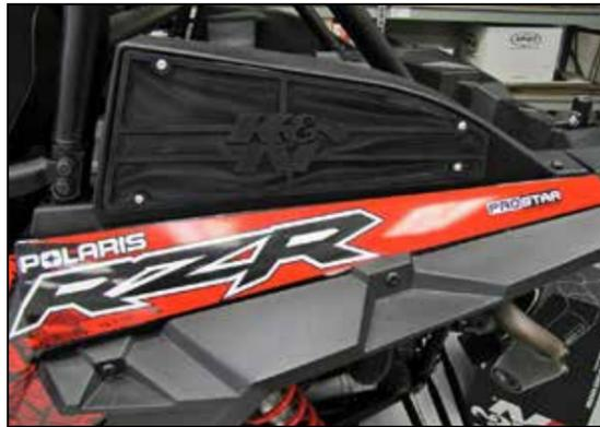
8. OPTION #2 Additional shorter hardware has been included so the pre-filters can be run without the scoops if desired. Be sure to use the cage supports for the pre-filter if the scoops are not used.
