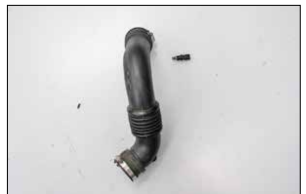
21. Remove the inlet air temperature sensor from the factory intake tube. NOTE: The inlet air temperature sensor is very fragile, use care while removing sensor.
