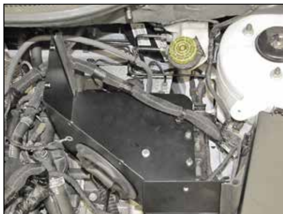
15. Install the heat shield onto the air box mounting plate so that the mounting stud installs into the grommet and the threaded studs protrude through the heat shield. Secure the heat shield with the provided hardware.
