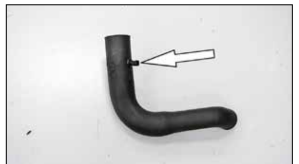
22. Install the inlet air temperature sensor into the grommet installed into the K&N® intake tube. NOTE: The inlet air temperature sensor is very fragile, use care while installing sensor.
