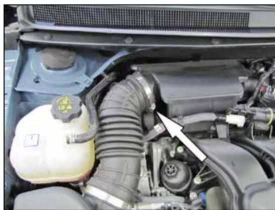
3. Loosen the hose clamp that secures the factory intake tube to the intake plenum.
