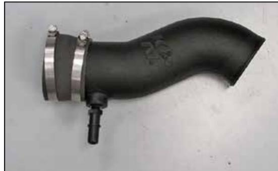
13. Install the provided quick disconnect npt fitting into the K&N® intake tube as shown.
