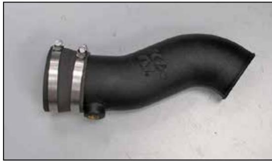
12. Install the provided coupler hose (084091) onto the K&N® intake tube fully but do not tighten at this time.
