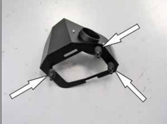
8. Install the mounting stud assemblies onto the heat shield and secure with the provided hardware.
