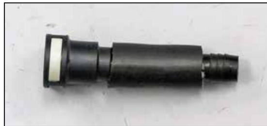
15. Remove the factory quick disconnect fitting from the factory crank case vent hose and install it into the provided vent hose as shown.
