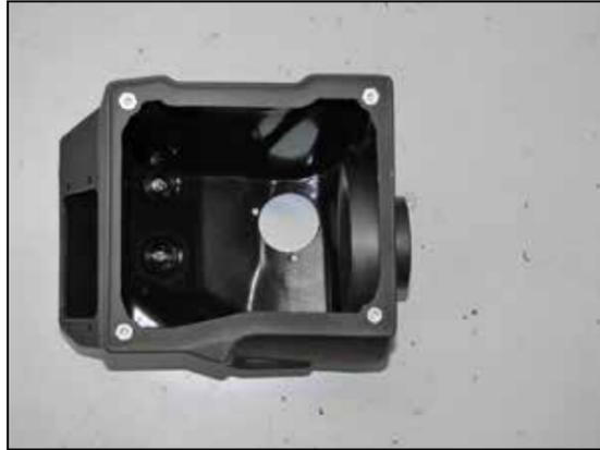
21. Using the provided hardware, secure the K&N® filter adapter to the air filter housing.
