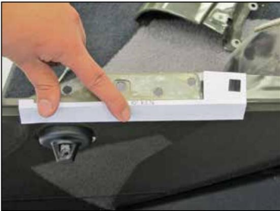
46. Using the provided template, mark the fender where the excess material needs to be removed from the fender.
