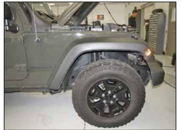
55. Reinstall the fender and secure with the factory hardware. Then reconnect the marker light and install the antenna mast.
