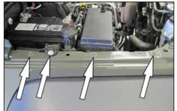
16. Remove the four bolts securing the top of the fender to the inner structure.
