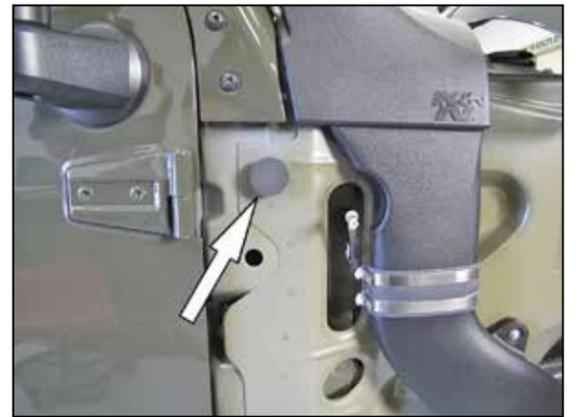
54. Peel the backing of the provided damper pad and then install it as shown on the inner body.
