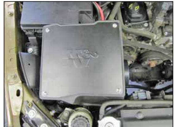
27. Install the air filter housing lid and gasket and secure with the provided hardware.
