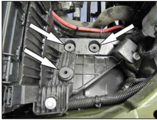
20. Install the provided insert nuts into the air filter housing mounting grommet locations.
