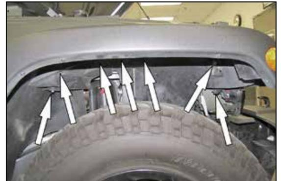
15. Remove the seven inner fender bolts.
