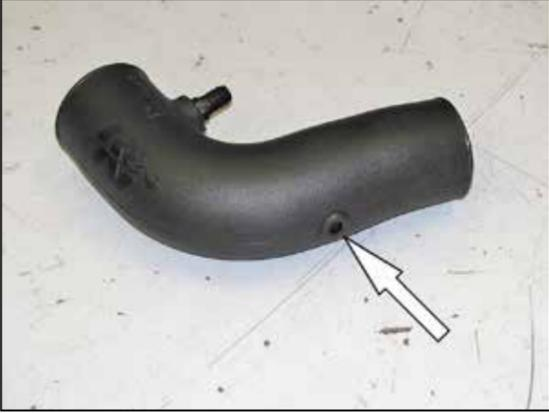
31. Install the provided grommet into the K&N® intake tube as shown.
