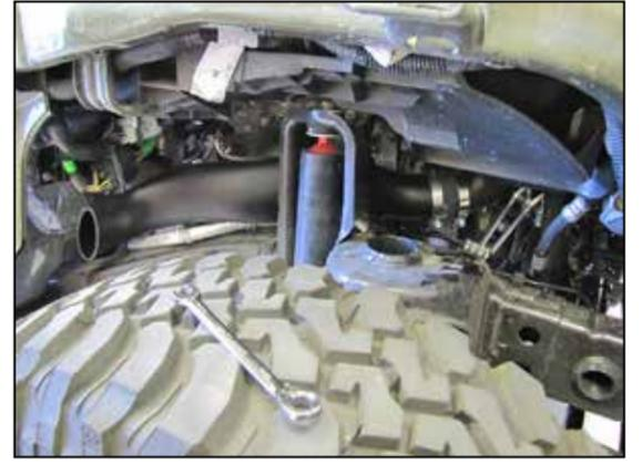
40. Install the lower tube into the coupler and align the mounting bracket with the nut extension. Secure the tube with the provided hose clamp and hardware.
