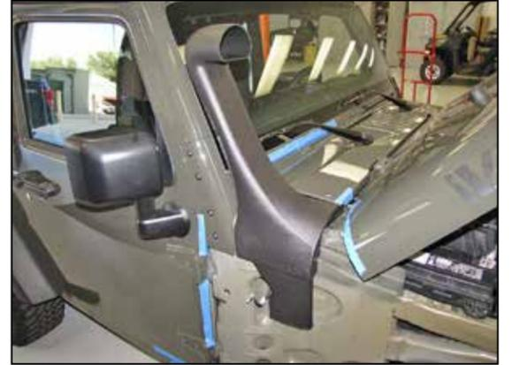
42. Temporarily install the snorkel and secure with the factory cowl bolts.
