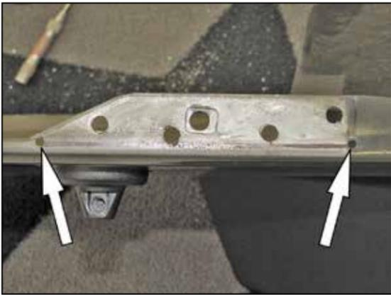
47. Drill a 3/16" id hole into each corner of the cut area as shown.
