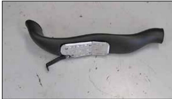
38. Install the provided heat shield and mounting bracket (064339) onto the K&N® lower tube as shown using the provided hardware.
