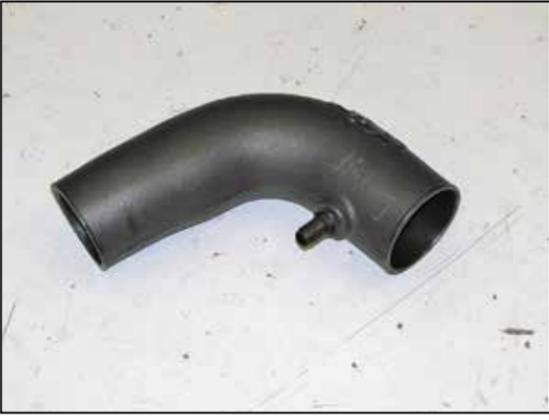
30. Install the provided NPT crank case vent fitting into the K&N® intake tube as shown.
