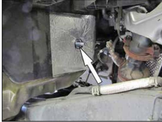
37. Install the provided nut extension and fender washer onto the stud as shown.
