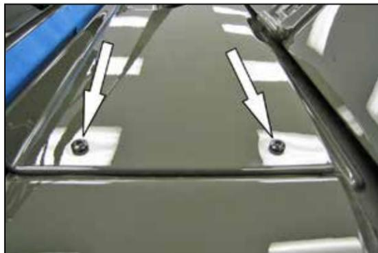
10. Using the T30 socket, remove the two bolts securing the cowl panel to the right side fender.
