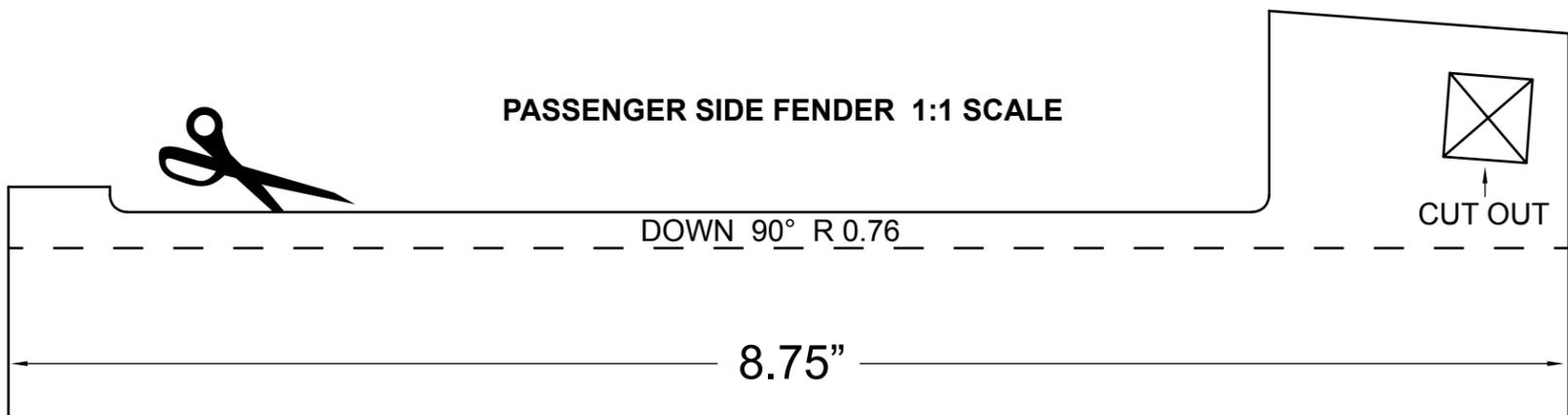
Carefully cut along outer edge of template and also cut out the square alignment hole.
