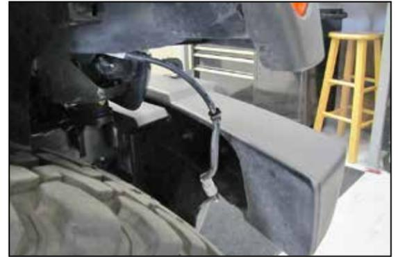
14. Remove the marker light bulb from the housing and disconnect the harness retaining clip from the fender.
