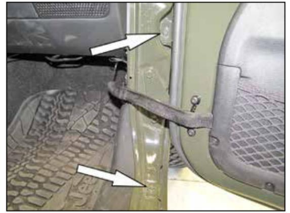
12. Loosen the two fender bolts inside the passenger door jamb.
