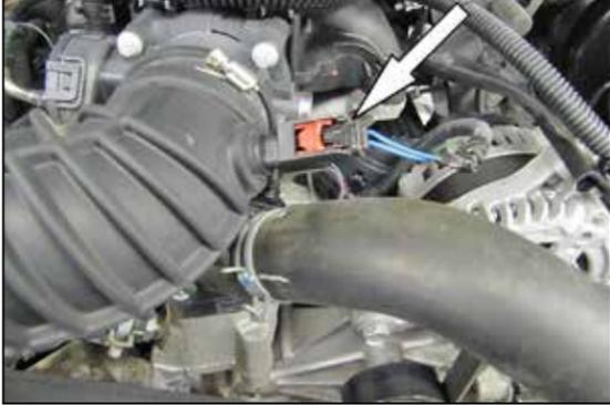
2. Release the red locking tab and then disconnect the inlet air temperature sensor electrical connection.
