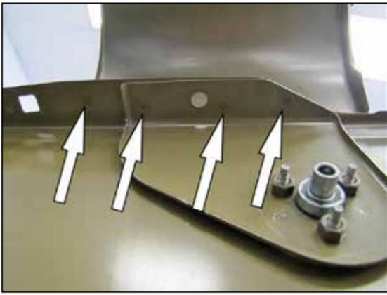
45. Use a center punch to mark the four spot welds which hold the cowl corner cap to the fender. Then drill out the spot welds to remove the cowl cap from the fender.
