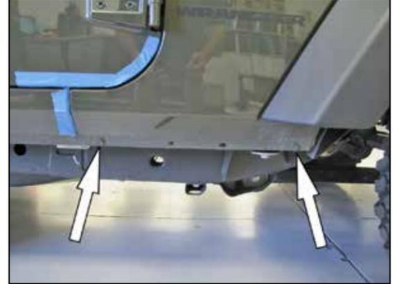
13. Remove the two lower fender bolts.
