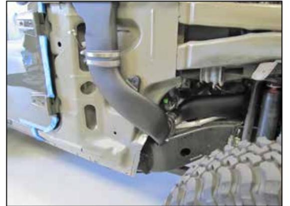
44. Install the provided coupler hose (08698) onto the corner tube, and then install the Corner tube assembly as shown, snug the hose clamps but leave them loose enough to provide adjustment.
