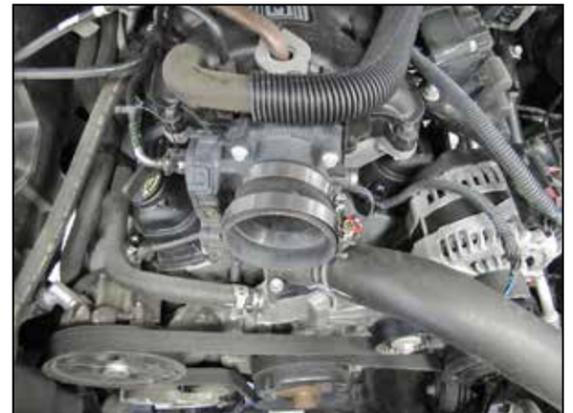
29. Install the provided coupler (084034) onto the throttle body and secure with the provided hose clamp.
