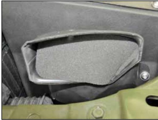
59. Use the provided dense foam to plug the fresh air intake duct when using in extreme wet conditions.
