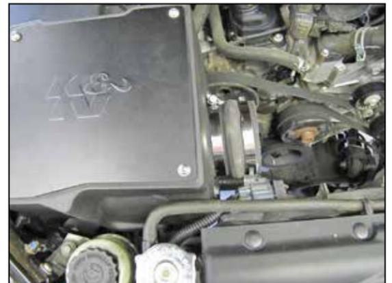
28. Install the provided hump coupler (08699) onto the filter adapter and secure with the provided hose clamp.
