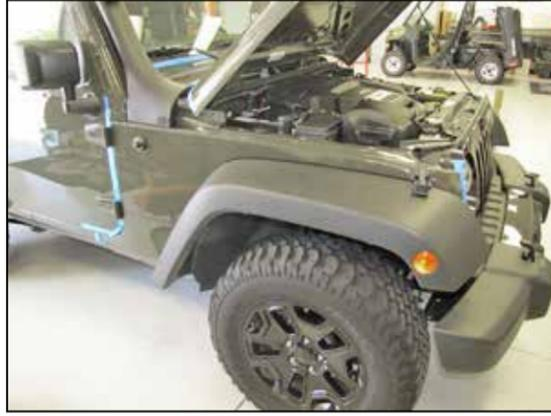
49. With an assistant, temporarily reinstall the fender onto the vehicle but do not secure it at this time. Adjust the snorkel for best fit and then secure the snorkel bracket to the inner cowl and the outer cowl to the snorkel with the factory hardware.
