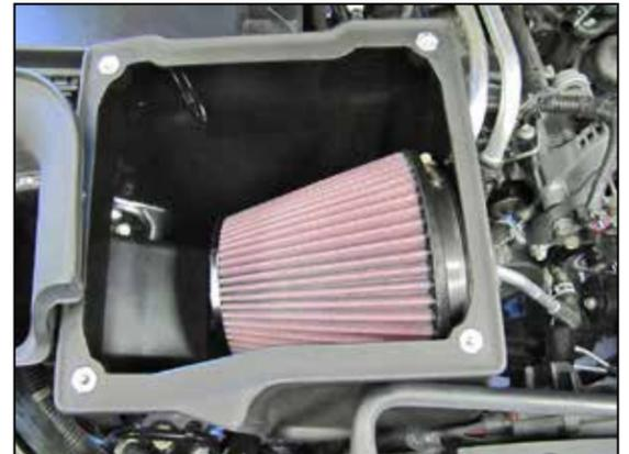
26. Install the K&N® air filter and secure with the provided hose clamp.
