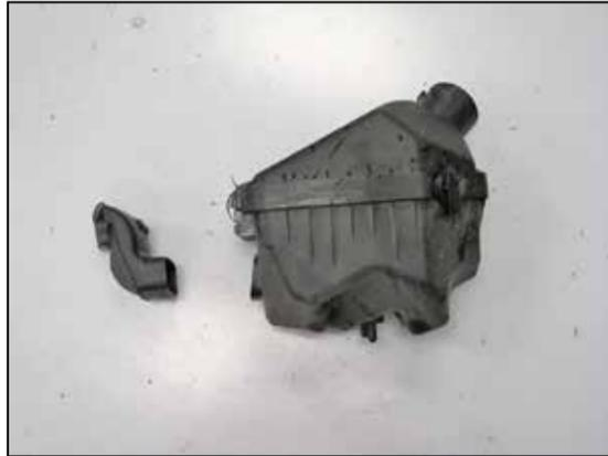
22. Remove the fresh air intake duct from the factory air filter housing.
