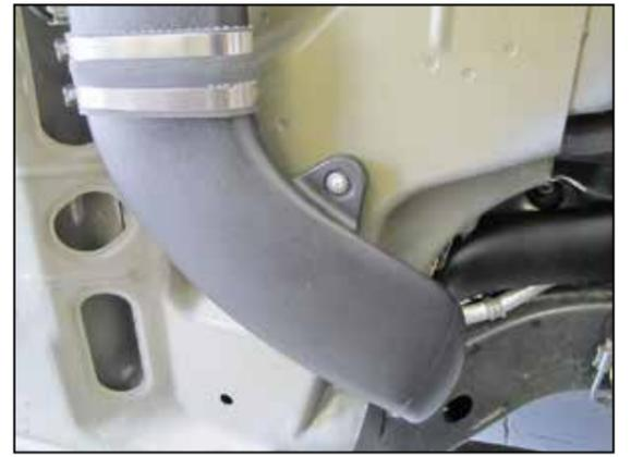
52. Secure the corner tube with the provided sheet metal screw into the hole previously drilled.
