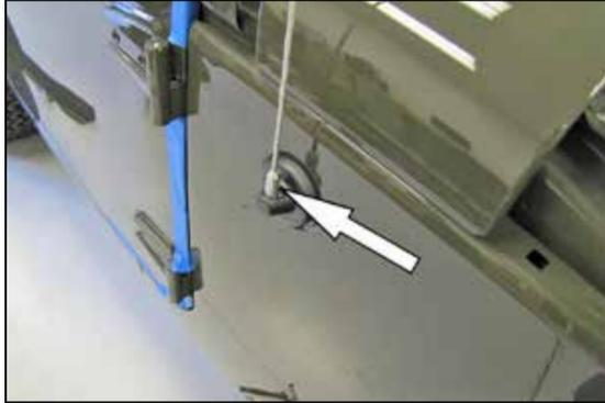
8. Remove the antenna mast.
