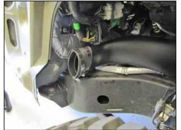
43. Install the provided coupler hose (08711) onto the lower tube and secure with the provided hose clamp.
