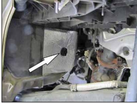
36. Remove the Insulation retaining nut shown.
