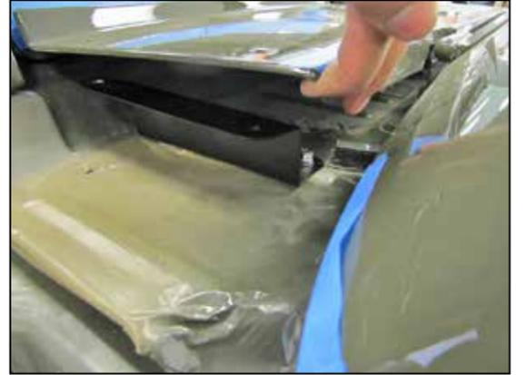
41. Install the snorkel mounting bracket (073219) onto the factory fender mounting points on the cowl using the provided hardware.
