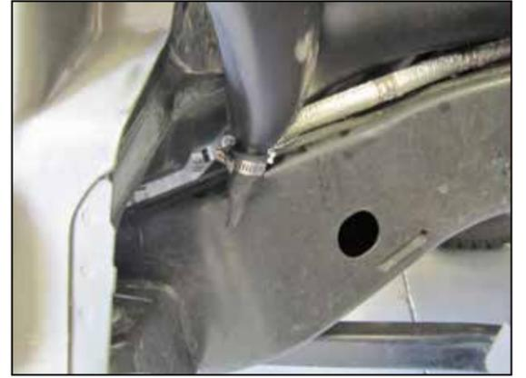
53. Install the duck bill fitting onto the port at the bottom of the corner tube and secure with the provided hose clamp.
