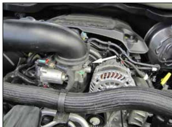
3. Loosen the hose clamp that secures the factory intake tube to the throttle body and then disconnect the intake tube from the throttle body.
