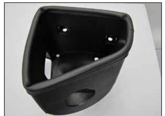
5. Install the provided edge trim onto the K&N® air filter housing as shown.
