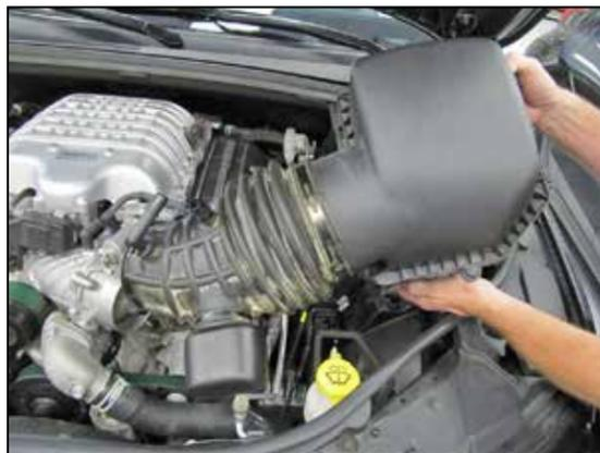
4. Lift the air filter housing assembly up to release it from the mounting grommets and then remove the complete intake system from the vehicle.
