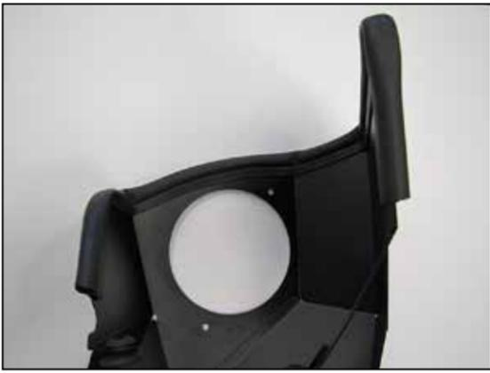
7. Install the provided edge trim onto the heat shield as shown.
