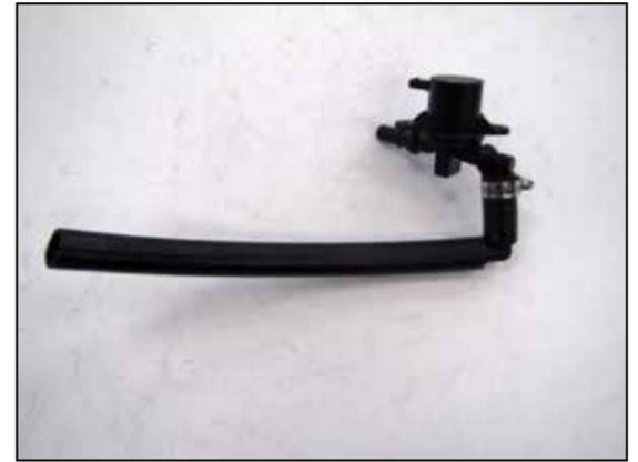
14b. remove the O-ring from the valve and then assemble the provided  $\frac{3}{4}$ " hoses and 90deg. Union as shown. Secure the hose to the valve with the clamp provided.
