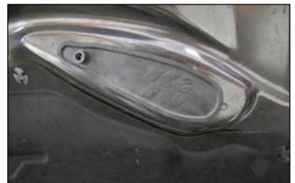
16. During wet conditions, install the provided hood vent block off to minimize water intrusion to the intake system. For Dodge vehicles, see step #17.
