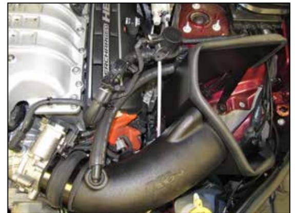
14c. Connect the factory CCV connector to the valve, route the  $\frac{3}{4}$ " hose to the fitting installed into the intake tube as shown. Using the mounting tree tie wrap, secure the valve to the heat shield.
