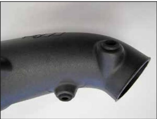
10. Install the provided grommets into the K&N intake tube as shown.
