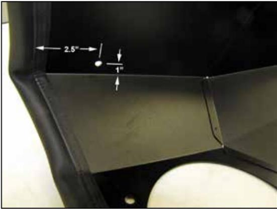
7a. On vehicles equipped with the CCV valve on the air filter housing lid, drill a  $\frac{1}{4}$ " id hole 2.5" down from the top of the heat shield and 1.0" from the bend as shown. This hole will be used to secure the CCV valve to the heat shield.
