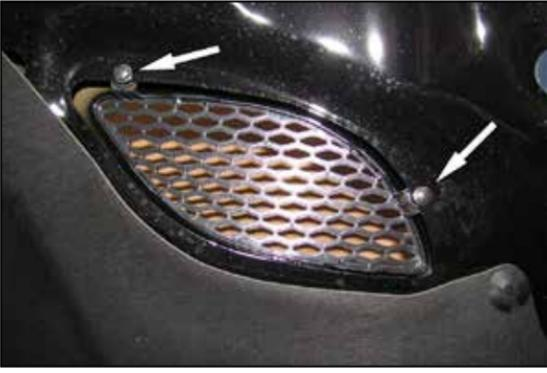
17. During wet conditions on Dodge vehicles to minimize water intrusion to the intake system, remove the two bolts that secure the heat extraction grill to the hood. Do not remove the grill.
