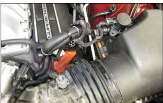
2a. On later models the CCV hose will connect to a valve on the air filter housing lid, disconnect the CCV hose and electrical connection at the valve.
