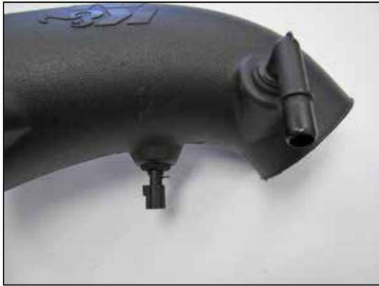
12. Remove the O-ring from the IAT sensor and then install the sensor into the K&N intake tube as shown. Install the factory quick connect CCV fitting into the K&N intake tube as shown.
