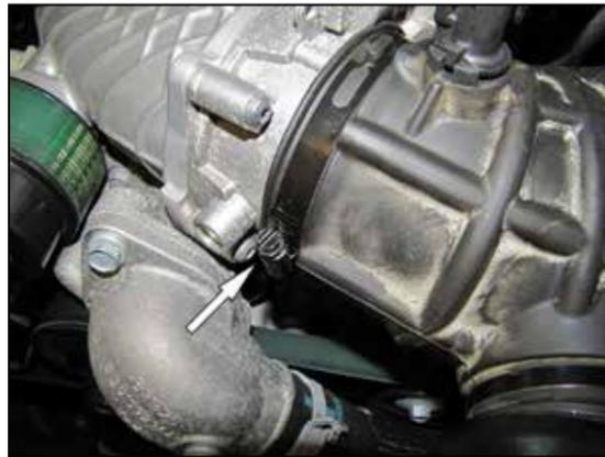
3. Loosen the hose clamp that secures the factory intake tube to the throttle body.
