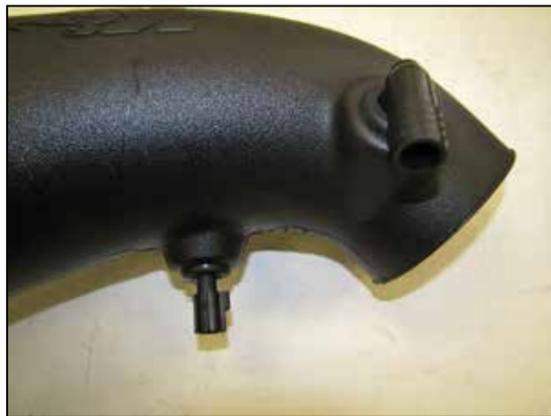
12a. On vehicles equipped with a CCV valve, install the provided 90deg union fitting into the K&N intake tube as shown.
