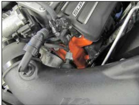
14. On vehicles not equipped with the CCV valve on the air filter housing lid, Reconnect the CCV quick connect fitting. Reconnect the IAT sensor electrical connection.
