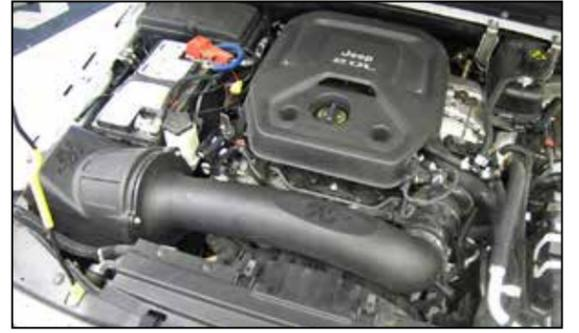
17. Install the intake assembly into the vehicle so the mounting studs insert into the mounting grommets and the intake tube inserts into the coupler. Secure the system with the provided hose clamp and hardware.
