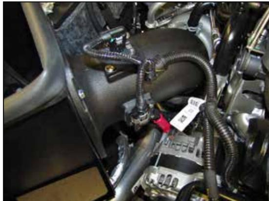
14. Install the intake tube assembly onto the turbo inlet and into the heat shield. Secure the tube with the provided hose clamp and hardware. Reconnect the air sensor electrical connection.
