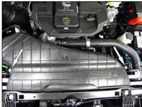
3. Remove the two bolts that secure the fresh air inlet duct to the core support and then remove the inlet from the vehicle.
