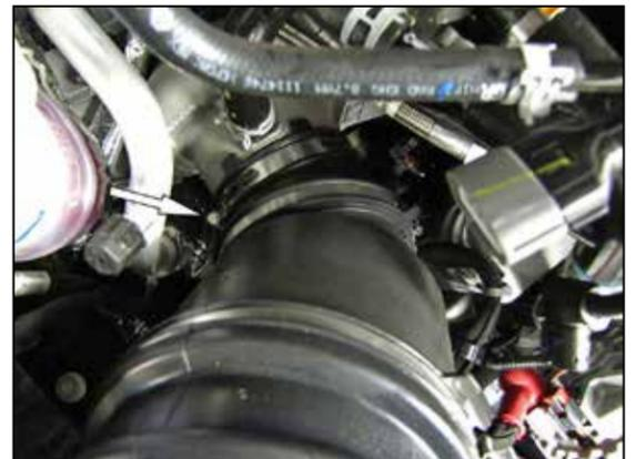
6. Loosen the hose clamp that secures the factory intake tube to the turbo inlet and then remove the tube from the vehicle.
