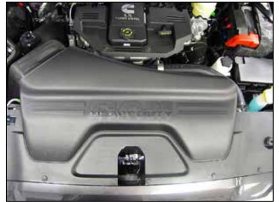
17. Reinstall the factory core support cover and secure with the factory retaining clips.
