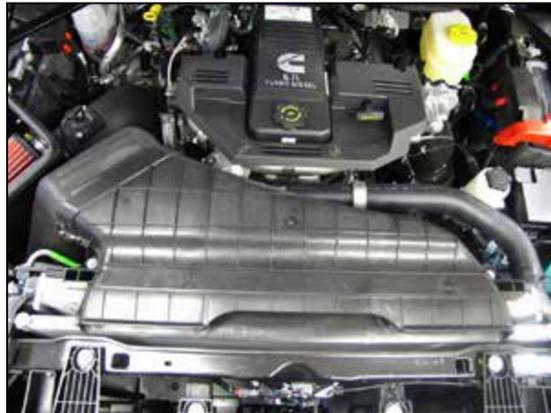
16. Install the K&N® fresh air duct into the heat shield and then install the factory portion of the fresh air duct and secure with the factory hardware.
