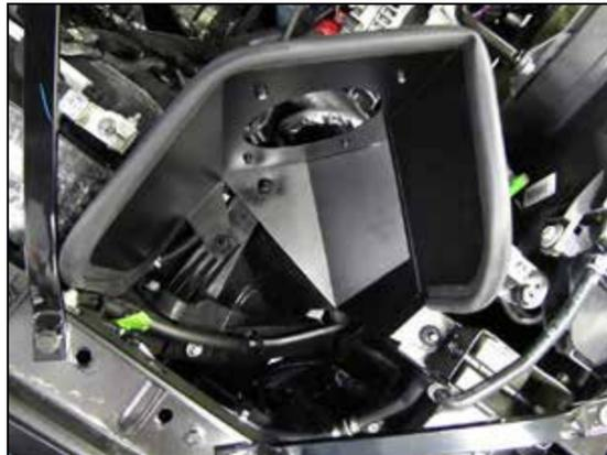
13. Install the heat shield assembly into the vehicle so the factory mounting posts protrude through the mounting grommets.
