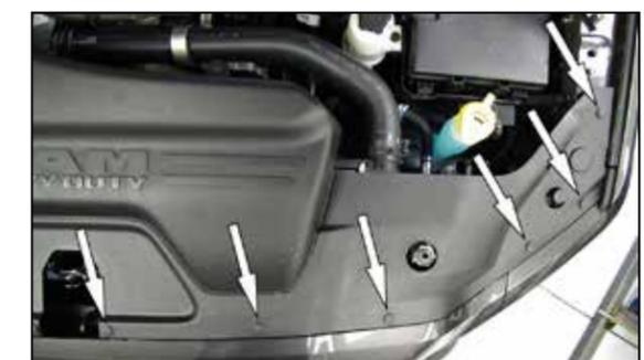
2. Remove the 14 push clips that secure the upper core support plastic cover and then remove the cover from the vehicle.
