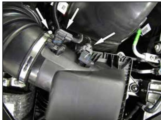
4. Loosen the hose clamp that secures the intake tube to the air filter housing and disconnect the electrical connections of the two air sensors.
