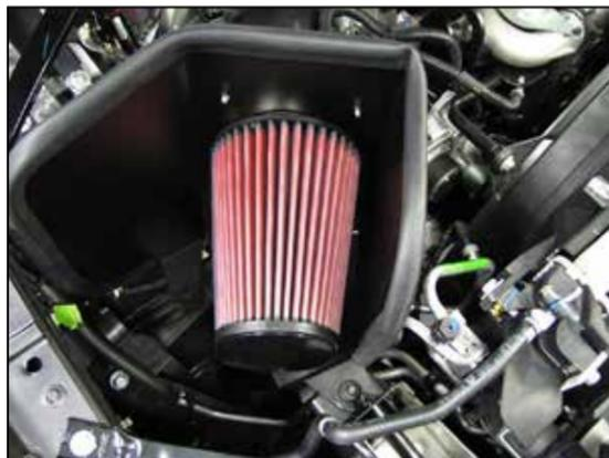
15. Install the air filter onto the intake tube and secure with the provided hose clamp.
