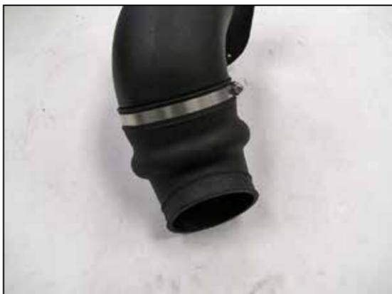
10. Install the flex coupler onto the intake tube and secure with the provided hose clamp. The coupler is keyed and can only be install in one location.
