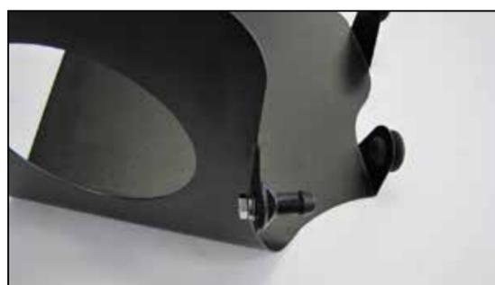
6. Install the air box mounting stud onto the K&N® heat shield using the provided hardware.
