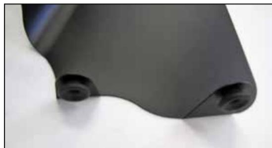
5. Remove the two factory mounting grommets from the factory air filter housing and install them into the K&N® heat shield as shown.
