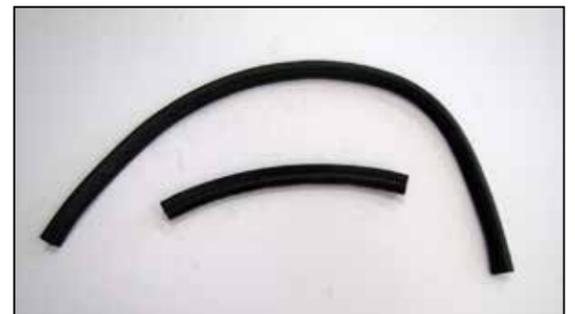
7. Cut the provided edge trim into two sections, 36" and 13.5" as shown.
