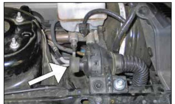
5. Install the provided cap onto the drum as shown.
