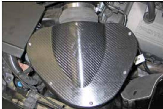
30. Install the K&N® airbox lid and secure with the provided hardware.
