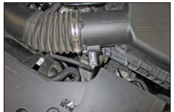
6. Unhook the mass air sensor electrical connection.
