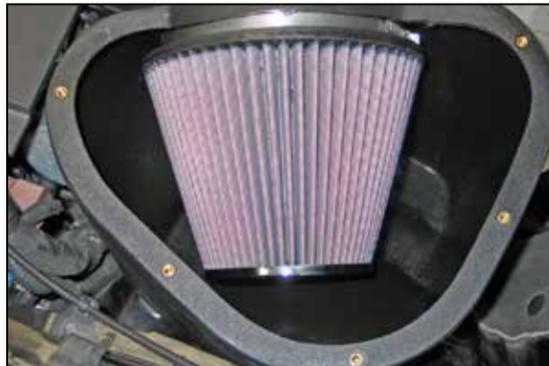
29. Install the K&N® air filter onto the filter adapter and secure with the provided hose clamp.
