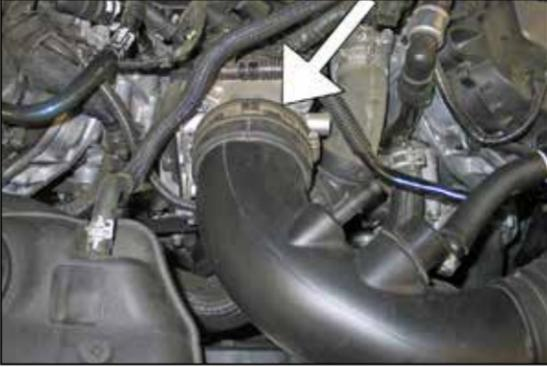
8. Loosen the hose clamp that secures the factory intake tube to the throttle body.
