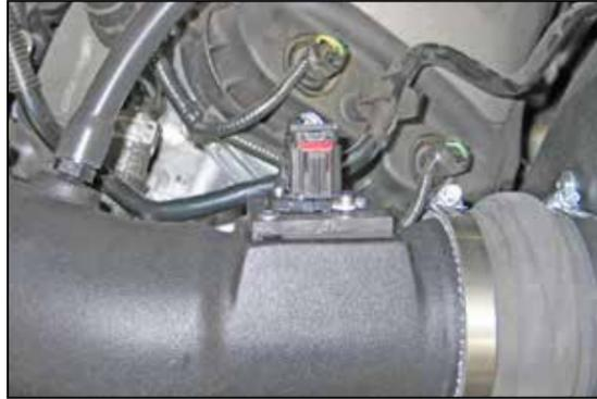
28. Reconnect the mass air sensor electrical connection.
