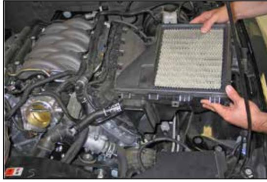
12. Remove the lower airbox from the vehicle.
