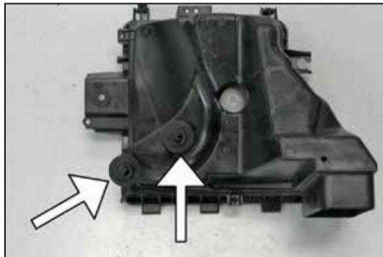
15. Remove the two airbox mounting grommets from the factory airbox.
