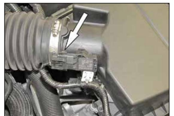
6. Disconnect the temperature sensor electrical connect.
