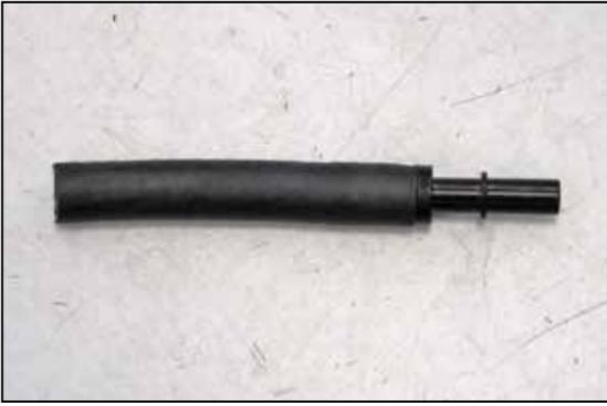
22. On 2014-15 model year vehicles, install the provided EVAP vent hose onto the provided quick disconnect union as shown.
