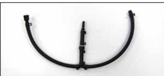
24. Cut the 5" hose in half and assemble the new EVAP hose assembly as shown, note the direction of flow of the check valve and install the flow restrictor as indicated.
