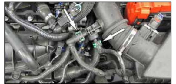
4a. On vehicles with an EVAP tee, unlock the two green locking tabs and then disconnect the EVAP lines from the intake tube. Release the green locking tab and disconnect the EVAP line that also connects to the intake charge pipe near the turbo. **NOTE: follow the vent line down towards the turbo to locate the connection.**
