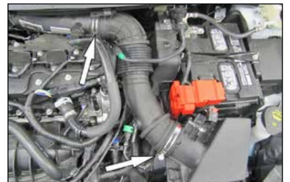
5. Loosen the hose clamps securing the factory intake tube to the turbo inlet pipe and to the factory air filter housing. Remove the factory intake tube from the vehicle.
