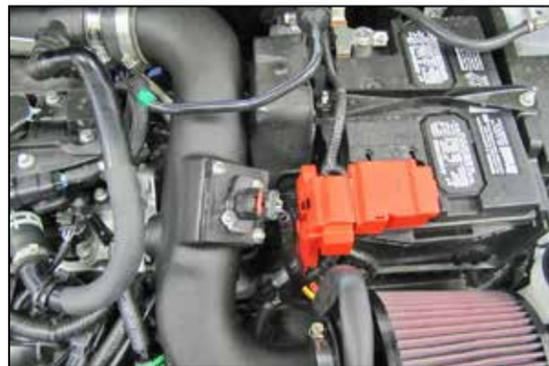
27. Connect the mass air sensor electrical connection as shown.
