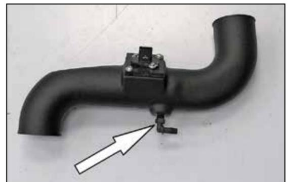
20. Install the 90° vent fitting into the K&N® intake tube as shown.
