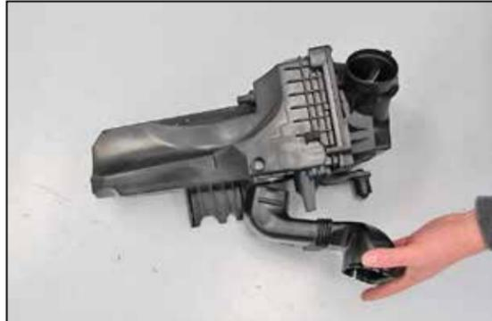
13. Remove the fresh air intake duct from the factory air box by pulling it away.
