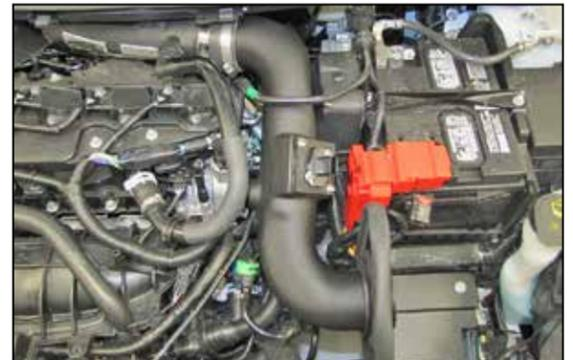
21. Install the K&N® intake tube assembly into the silicone hose at the turbo inlet pipe and then into the heat shield, adjust the tube for proper fit and then secure with the provided hose clamps.
