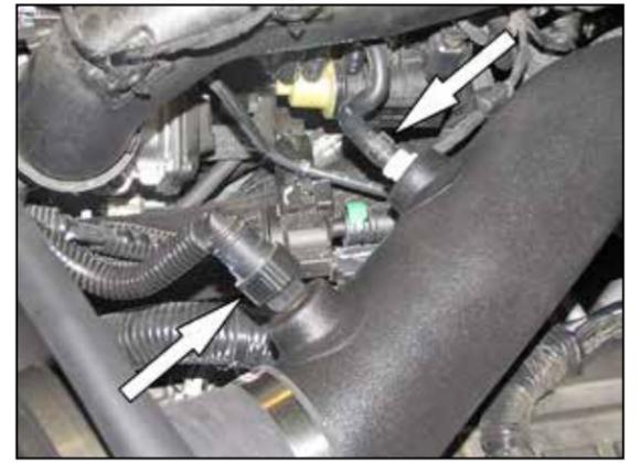
22. Connect the factory solenoid vent hose and the factory crank case vent hose to the fittings installed into the K&N® intake tube.
