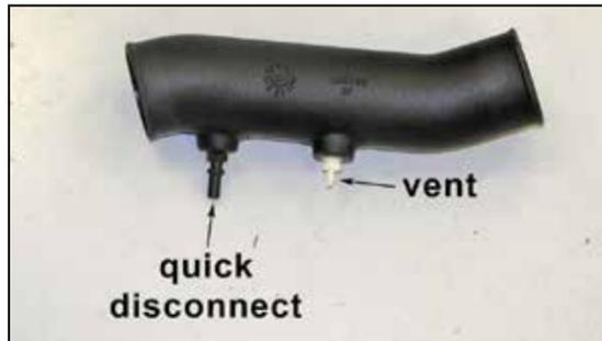
18. Install the provided 1/4" npt fittings into the K&N® intake tube as shown.
