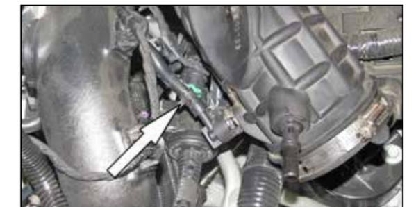
7. Loosen the hose clamp securing the factory intake tube to the turbo and then remove the hose from the vehicle.
