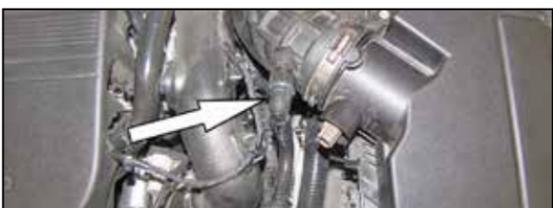
3. Disconnect the crank case vent hose from the factory intake tube.
