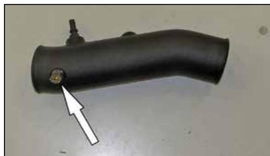
20. Install the provided grommet into the K&N® tube then install the inlet air temperature sensor into the grommet.
