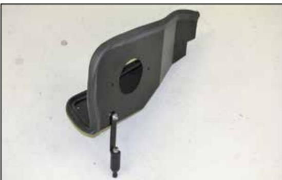
12. Install the mounting bracket assembly onto the heat shield as shown using the provided hardware.
