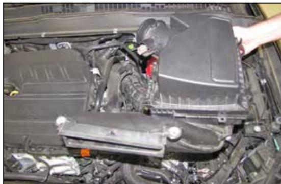
6. Lift up the air box to dislodge it from the mounting grommets and then remove it from the vehicle.
