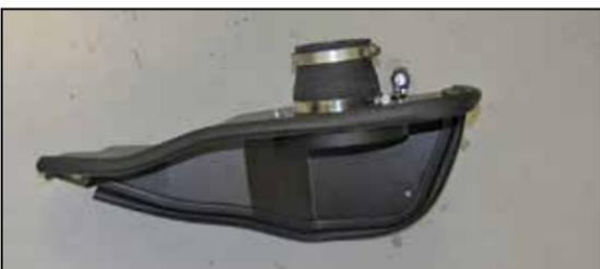
14. Install the provided step coupler (084055) onto the filter adapter and secure with the provided hose clamp.
