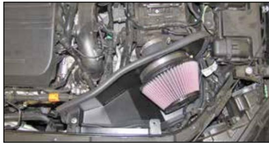
16. Set the heat shield assembly into the vehicle. The mounting stud will insert into the factory air box mounting grommet and the front of the heat shield will be secured to the core support with the provided hardware.
