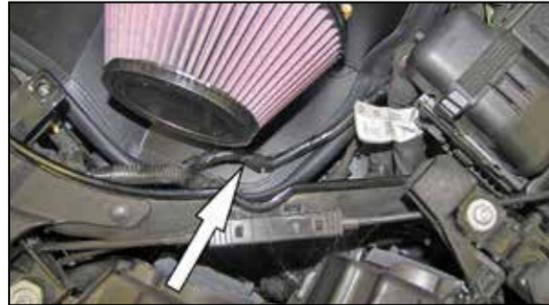
17. Clip the inlet air temperature sensor harness into the hole provided in the heat shield.
