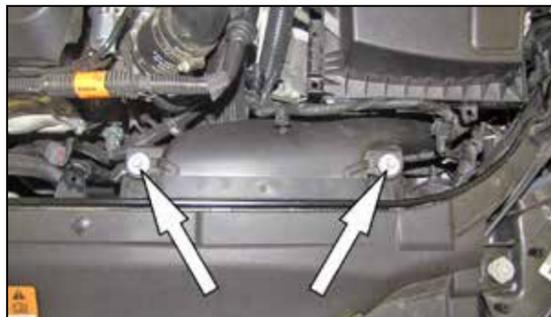
5. Remove the two bolts securing the fresh air intake scoop.
