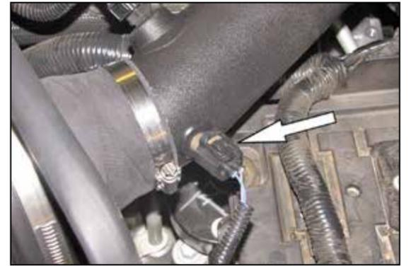
23. Using the provided extension harness, connect the inlet air temperature sensor electrical connection.
