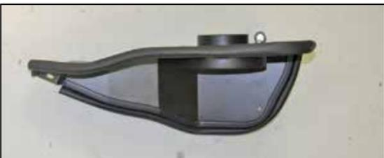
13. Install the filter adapter into the heat shield and secure with the provided hardware.
