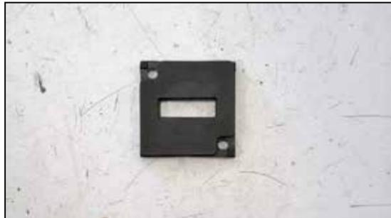
13. Install the provided gasket onto the K&N® mass air sensor adapter.
