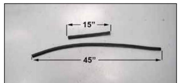
6. Cut the provided edge trim into two lengths, one should be 15" long and the other should be 45" long.
