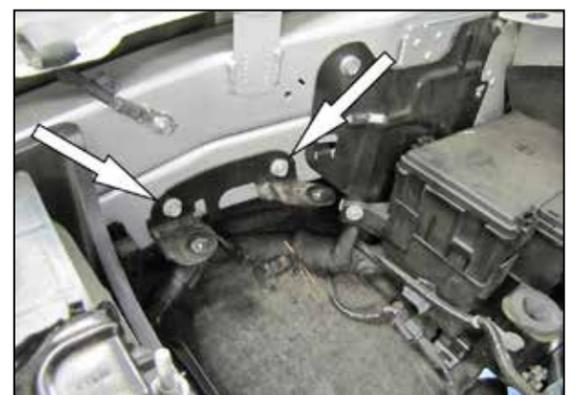
5. Remove the two bolts shown that secure the air filter housing bracket to the inner fender and then remove the bracket from the vehicle.
