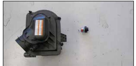
17. Remove the factory filter minder from the air filter housing.
