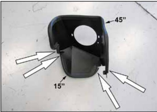
7. Install the edge trim onto the heat shield as show.
