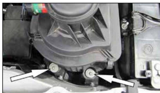
4. Remove the two filter housing mounting bolts shown and then remove the complete air filter housing from the vehicle.
