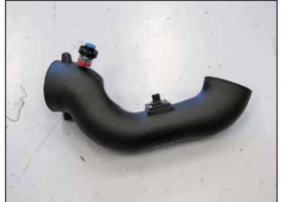
18. Install the filter minder using the provided grommet into the K&N® intake tube.
