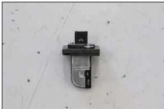
15. Install the sensor into the K&N® mass air sensor adapter and secure with the provided hardware.
