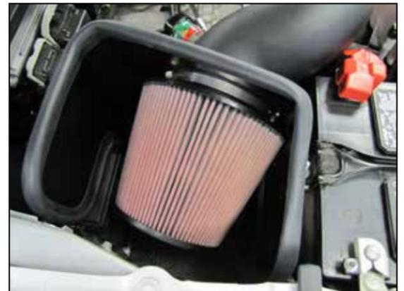
20. Install the K&N® air filter onto the intake tube and secure with the provided hose clamp.
