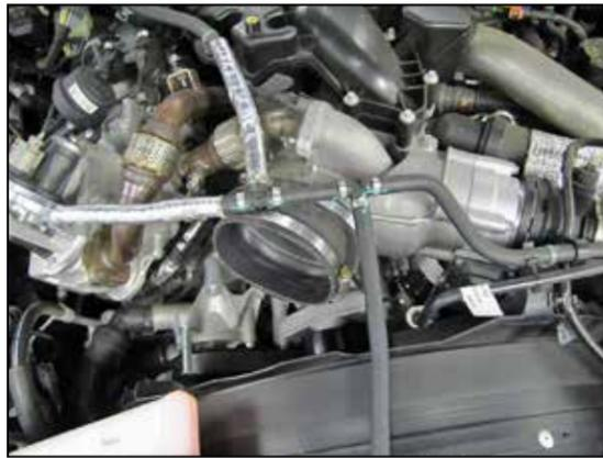
12. Install the provided coupler hose (08695) onto the turbo inlet and secure with the provided hose clamp.
