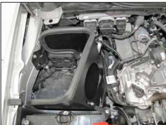
11. Install the heat shield into the vehicle so that the mounting studs insert into the factory air filter housing mounting grommets.
