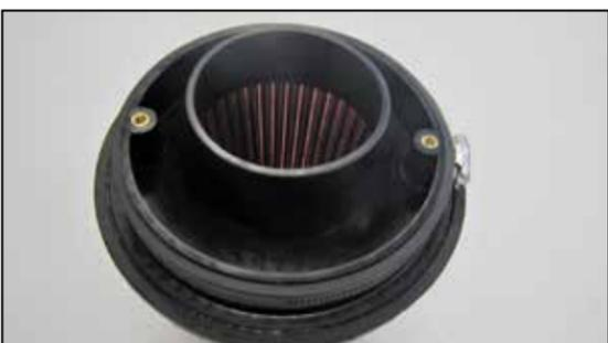
12. Install the filter adapter into the K&N® air filter.
