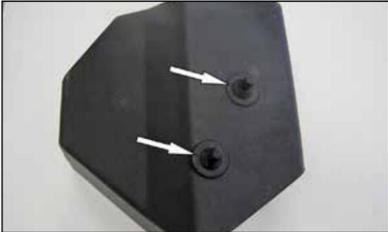
8. Install the two mounting studs provided into the K&N® lower air filter housing.
