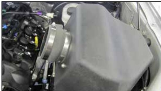
15. Install the provided hump coupler (08639) onto the filter adapter and secure with the provided hose clamp.
