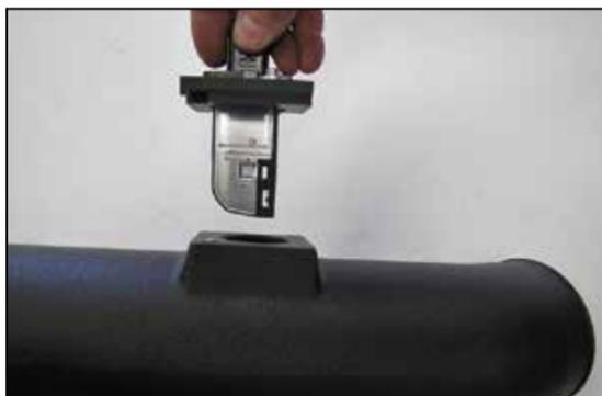
17. Install the mass air sensor assembly into the K&N® intake tube as shown using the provided hardware.
