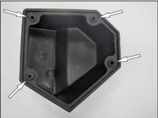
9. Install the four mounting grommets into the K&N® lower air filter housing.
