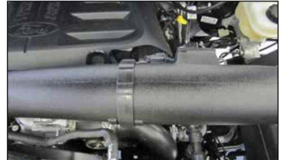
20. Secure the mass air sensor wiring harness to the K&N® intake tube.
