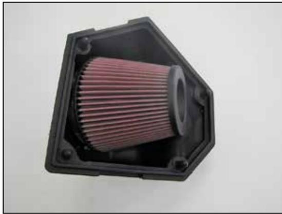
13. Install the K&N® air filter assembly into the upper housing using the provided hardware..
