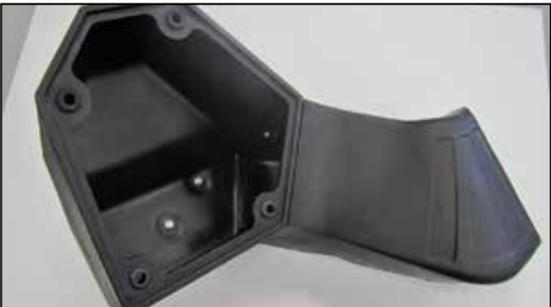
10. Secure the K&N® fresh air intake duct to the lower air filter housing using the hardware provided.
