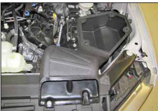
11. Install the K&N® air filter housing assembly into the vehicle so the mounting studs insert into the factory mounting grommets and then secure with the bolt and retaining clips provided.
