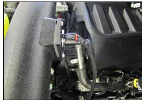
19. Use the provided extension harness to connect the mass air sensor electrical connection.
