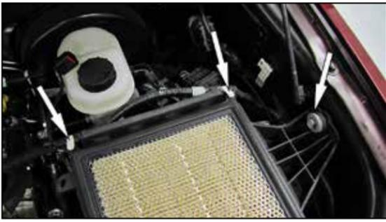
7. Disconnect the mass air sensor wiring harness from the lower air filter housing. Remove the bolt that secures the lower air filter housing to the inner fender and then remove the lower housing from the vehicle.
