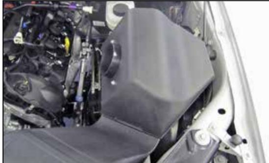
14. Install the upper filter housing assembly onto the previously installed lower housing so the mounting studs insert into the grommets.
