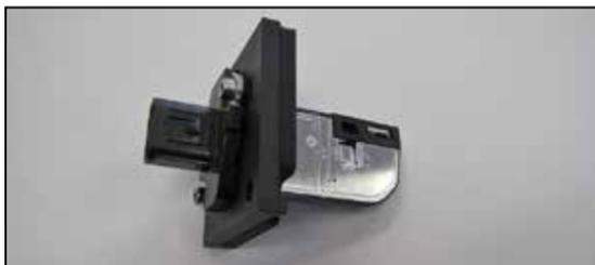
16. Remove the mass air sensor from the factory air filter housing. Assemble the mass air sensor, gasket and adapter as shown using the provided hardware.
