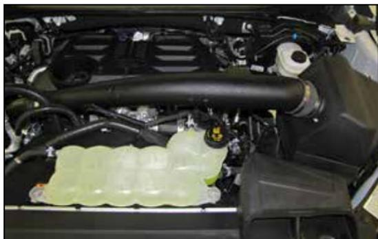
18. Install the K&N® intake tube assembly into the couplers, adjust for best fit and then secure with the hose clamps.
