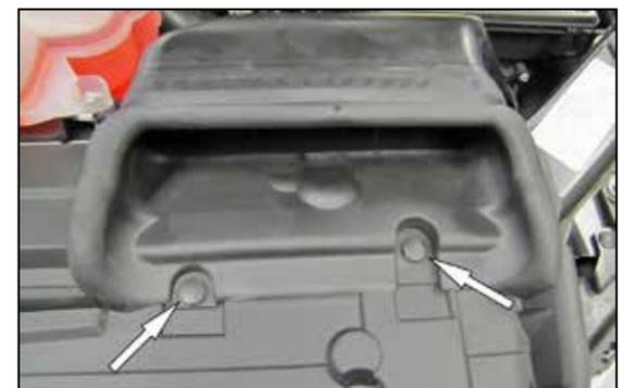
6. Remove the two clips that secure the fresh air intake duct to the core support.
