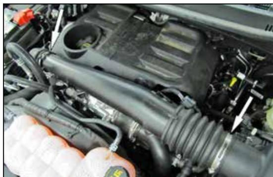
4. Loosen the two hose clamps that secure the factory intake tube and then remove the tube from the vehicle.
