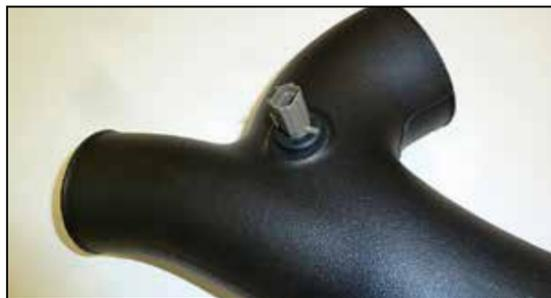
18. Remove the inlet air temperature sensor from the factory tube and remove the O-ring from the sensor. Using the provided grommet, install the inlet air temperature sensor into the K&N® intake tube.
