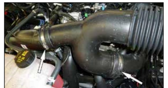
5. Loosen the hose clamps that secure the intake tube to the turbo inlet pipes and then remove the intake tube from the vehicle.
