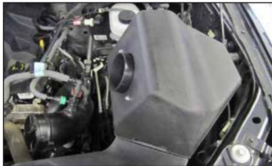
16. Install the upper filter housing onto the lower housing so the mounting studs insert into the mounting grommets.
