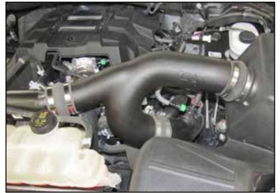
19. Install the K&N® intake tube into the couplers, align for best fit and then secure with the provided hose clamps.
