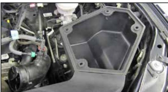
12. Install the K&N® lower filter housing assembly into the vehicle so the mounting studs insert into the factory mounting grommets. Secure the filter housing with the hardware provided to the rubber mounted stud.
