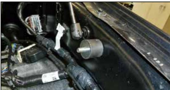
11. Install the provided rubber mounted stud into the factory filter housing mounting location as shown.
