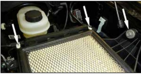
7. On vehicles that have the wiring harness and purge solenoid attached to the lower air filter housing disconnect them from the housing. Remove the bolt that secures the lower housing to the inner fender and then remove the housing from the vehicle.
