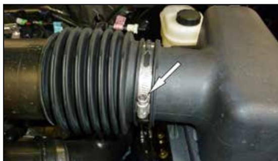
3. Loosen the hose clamp that secures the factory intake tube to the upper air filter housing.
