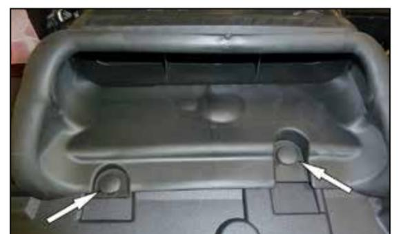
6. Remove the two clips that secure the fresh air intake duct to the core support.
