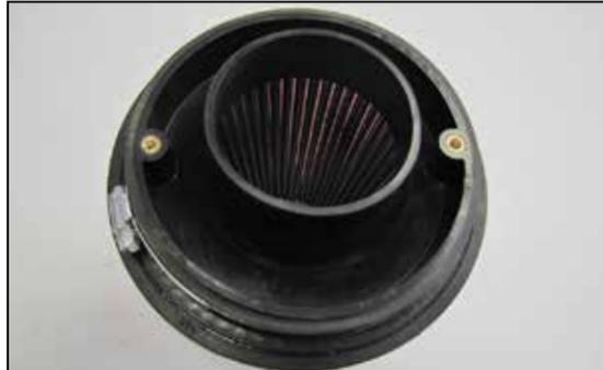
14. Install the filter adapter into the filter and secure with the provided hose clamp.
