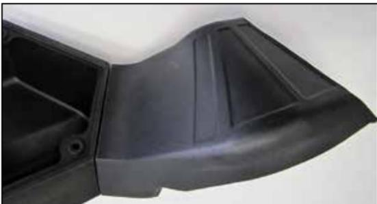
10. Attach the K&N® fresh air intake duct to the lower housing using the provided hardware.
