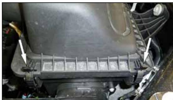
4. Release the two clips that retain the upper air filter housing and then remove the upper housing from the vehicle.
