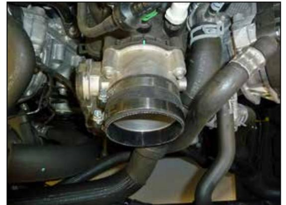
20. Install the provided coupler (08698) onto the throttle body and secure with the provided hose clamp.
