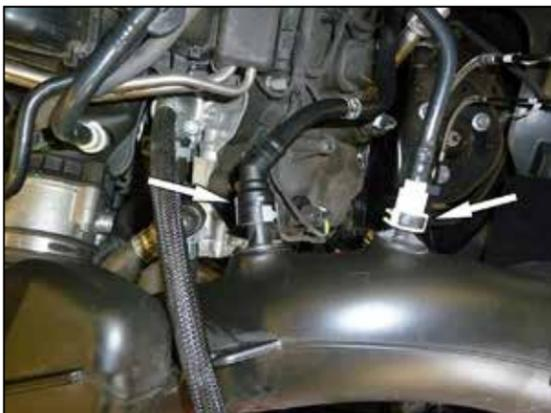
2. Depress the locking tabs and then disconnect the crank case vent and EVAP vent lines.
