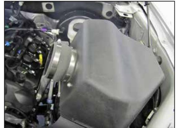
19. Install the provided hump coupler (08639) onto the filter adapter and secure with the provided hose clamp.
