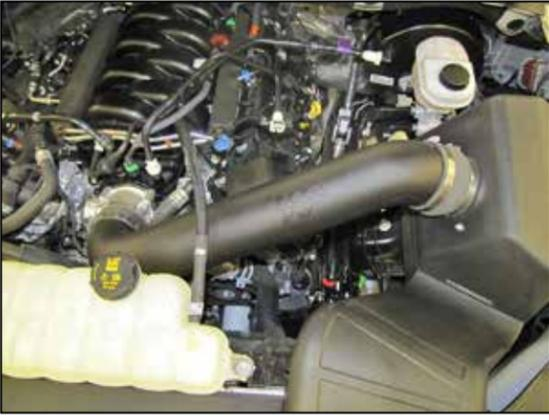
22. Install the K&N® intake tube into the couplers, adjust for best fit and then secure with the provided hose clamps.
