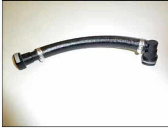
24. On vehicles that have the CCV hose connected to the valve cover between the second and third coil pack, assemble the provided CCV hose as shown.
