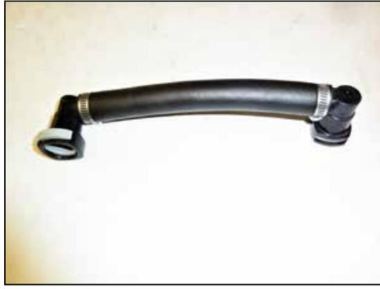
22. Assemble the provided CCV fittings and hose as shown.
