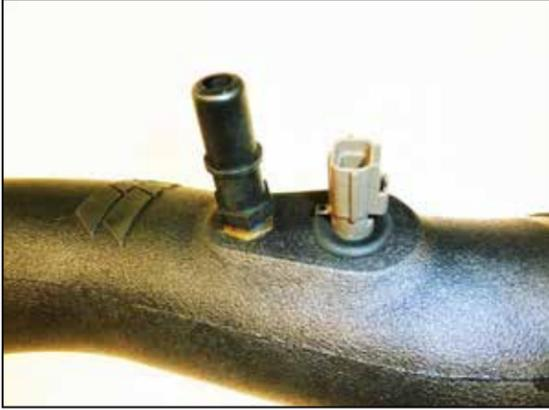
18. Remove the IAT sensor from the factory air filter housing, remove the O-ring from the sensor and then install the sensor into the K&N intake tube using the provided grommet. Install the provided CCV fitting into the K&N intake tube. **NOTE: The IAT sensor is fragile, use caution while handling the sensor.**
