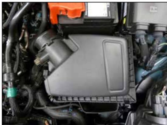
11. Lift up the factory air filter housing to dislodge it from the mounting grommets and remove it from the vehicle.
