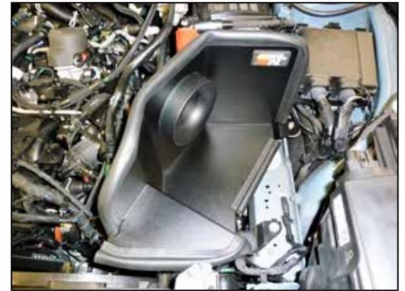
15. Install the heat shield into the vehicle so the mounting posts insert into the factory air filter housing mounting grommets.
