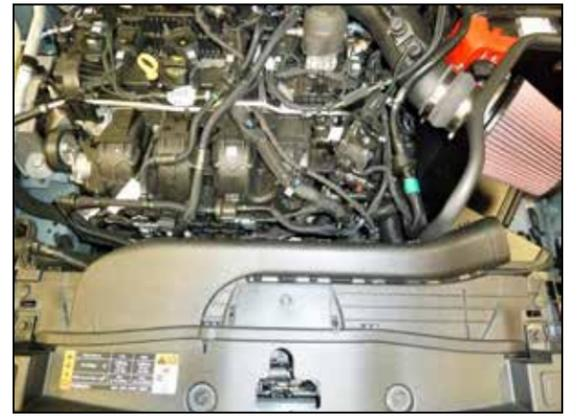
27. Reinstall the factory fresh air duct and secure with the factory pushpins.
