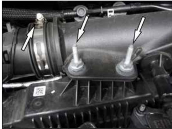
9. Loosen the hose clamp that secures the factory intake tube to the turbo inlet. Remove the hardware that secures the factory intake tube to the engine. This hardware will be reused with the K&N intake system.
