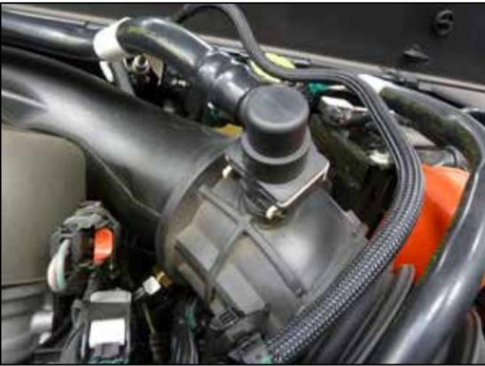
6. Release the white safety lock clip and then release the clip that secures the vent line to the factory intake tube and disconnect.
