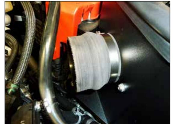
16. Install the provided hump hose onto the filter adapter and secure with the provided hose clamp.
