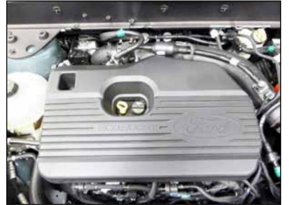
28. Reinstall the engine cover and secure with the factory hardware.
