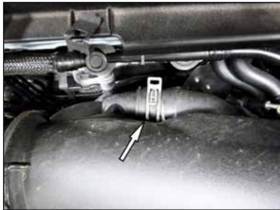
10. Release the spring clamp that secures the BOV hose to the factory intake tube and disconnect the BOV hose from the intake tube. Remove the complete stock intake tube from the vehicle.
