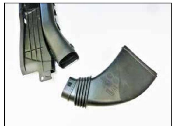
3. Separate the two sections of the fresh air intake duct, set the section that connects to the factory air box aside as it will not be used with the K&N intake system.
