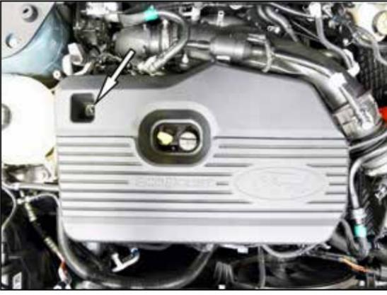
4. Remove the hardware that secures the engine cover and then remove the cover from the engine.
