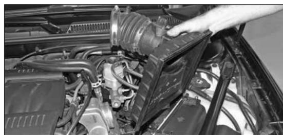
5. Remove the air box housing half and intake tube as shown.
