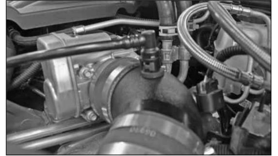
40. Reconnect the crank case vent tube to the vent fitting as shown.
