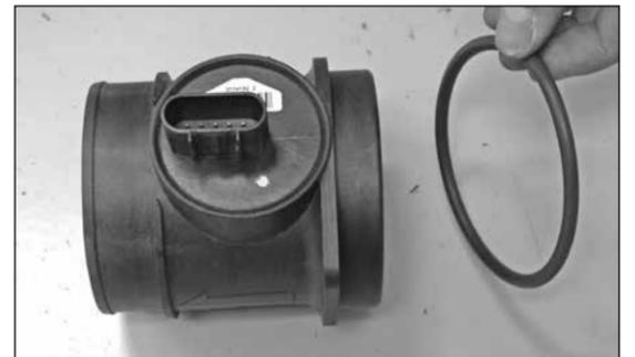
23. Remove the "O" ring from the mass air sensor as shown.
