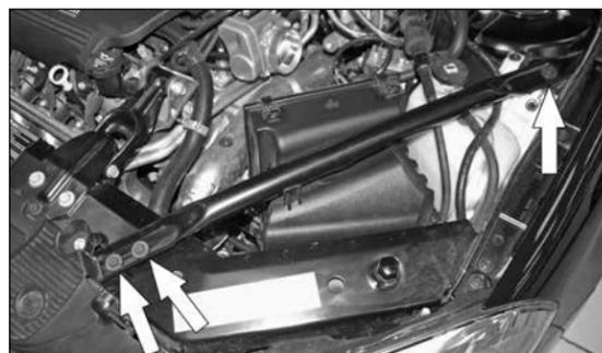
6. Remove the three body support brace mounting bolts shown and then remove the support brace from the engine compartment.
