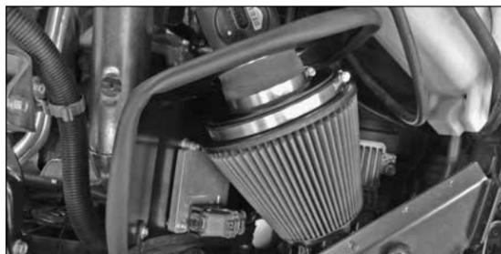
38. Install the air filter assembly onto the mass air sensor and secure with the provided hose clamp.
