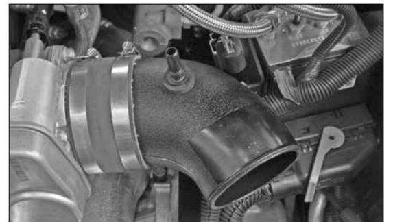
25. Install the K&N® intake tube into the silicone hose at the throttle body and align with the mounting bracket installed in step #17. Secure the silicone hose onto the throttle body with the supplied hardware and hose clamp.
