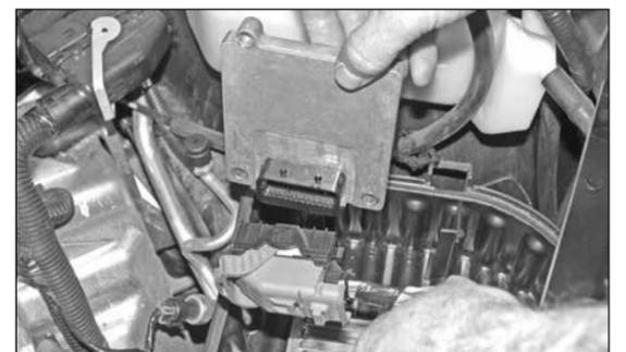
9. Remove the transmission control module from the housing, release the clamshell retaining clip, and then disconnect the wiring harness as shown.
