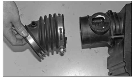
21. Loosen the hose clamp, which secures the stock intake tube to the mass air sensor, and then remove the hose from the sensor as shown.
