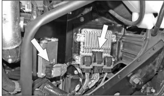
35. Reconnect the engine control module and transmission control module electrical connections.
