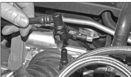
3. Release the locking tab and disconnect the crank case vent tube as shown.
