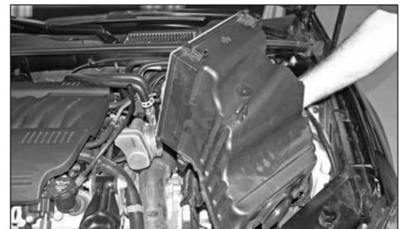
8. Remove the upper air box housing from the vehicle as shown.
