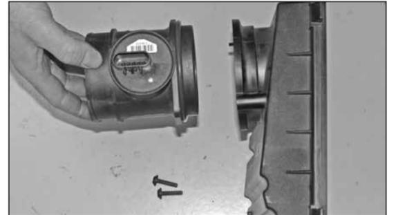
22. Remove the two screws, which secure the mass air sensor to the air filter housing and then remove the mass air sensor as shown.
