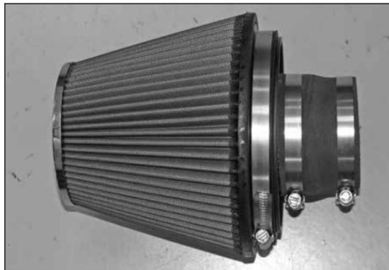
37. Install the silicone hose (08051) onto the K&N® filter assembly as shown and secure with the provided hose clamp.
