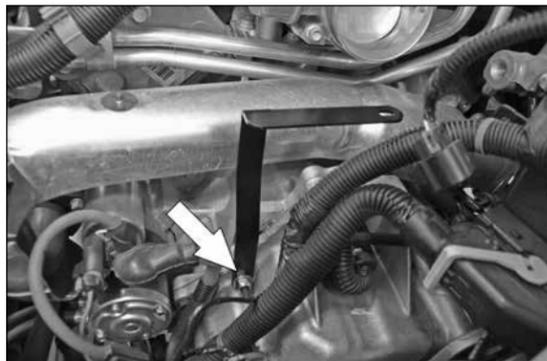
17. Install the tube mounting bracket (26627) onto the existing transmission stud as shown.
