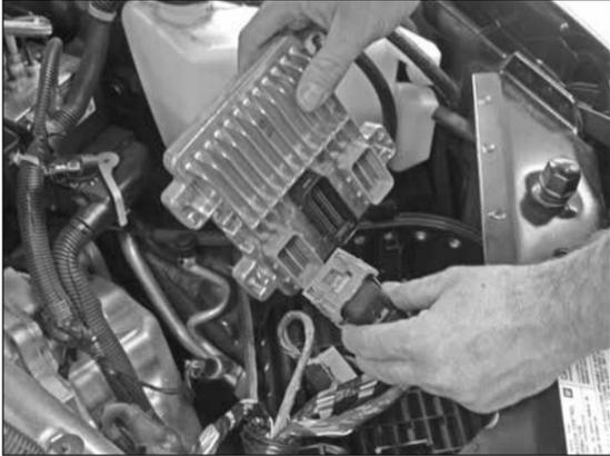
11. Release the engine control module wiring harness clamshell clips and disconnect the wiring harness from the engine control module.
