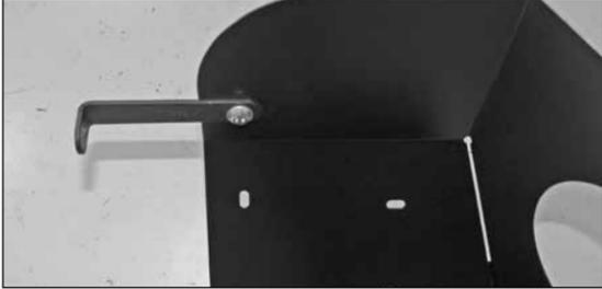
28. Install the mounting bracket (070952) onto the heat shield with the provided hardware.
