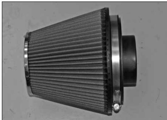
36. Install the filter adapter into the K&N® air filter as shown and secure with the provided hardware.
