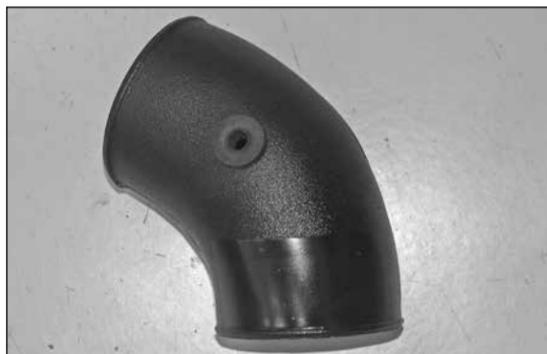
19. Install the provided grommet into the K&N® intake tube as shown.
