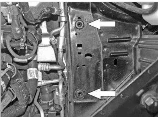
13. Remove the two mounting grommets shown from the inner fender.
