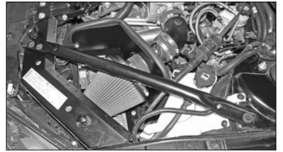
39. Reinstall the body brace removed in step #6 and secure with the factory bolts.
