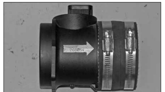
26. Install the silicone hose (08690) onto the mass air sensor as shown and secure with the provided hose clamps.
