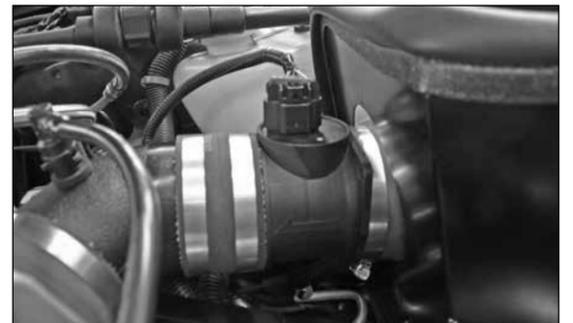
41. Reconnect the mass air sensor electrical connection.
