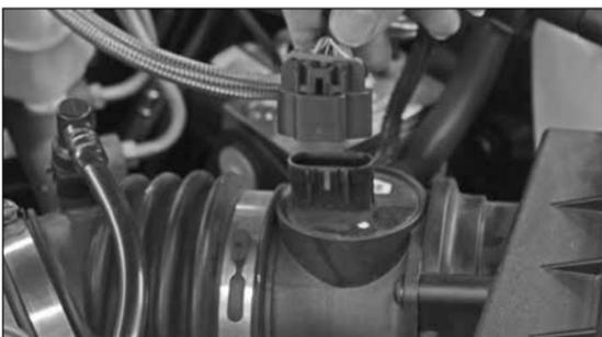
2. Depress the locking tab on the mass air sensor electrical connection, then disconnect the mass air sensor electrical connection as shown.
