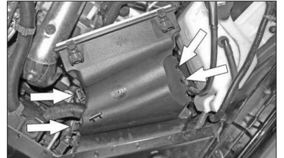
7. Depress the four air box housing retaining clips shown.
