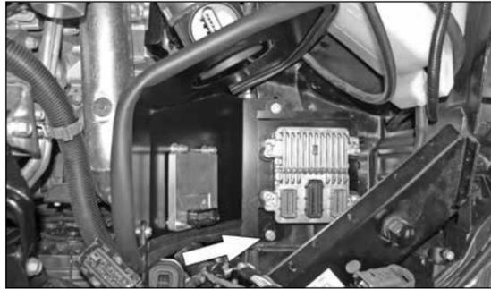
34. Place the engine control module assembly into position on top of the heat shield, then secure the heat shield and control module bracket to the inserted nuts installed in step #31 with the provided hardware.
