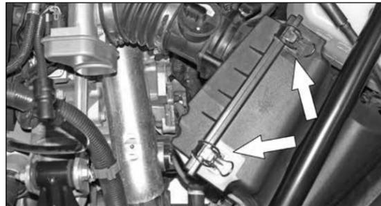
4. Loosen the hose clamp, which secures the intake tube to the throttle body, and release the air box over center clips shown.
