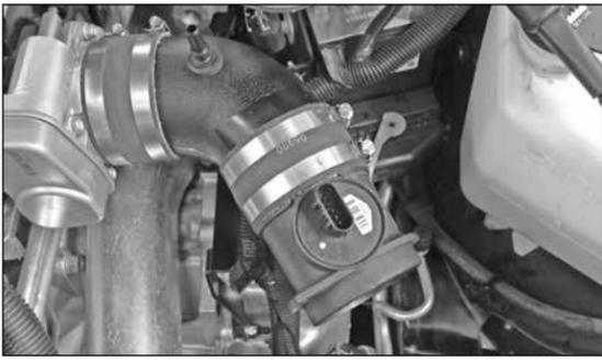
27. Install the mass air sensor assembly onto the K&N® intake tube as shown and secure with the provided hose clamp.
