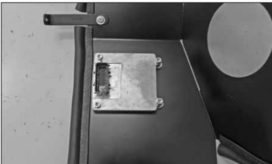
30. Secure the transmission control module to the heat shield with the provided hardware as shown.
