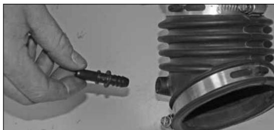
20. Remove the crank case vent fitting from the stock intake tube as shown.
